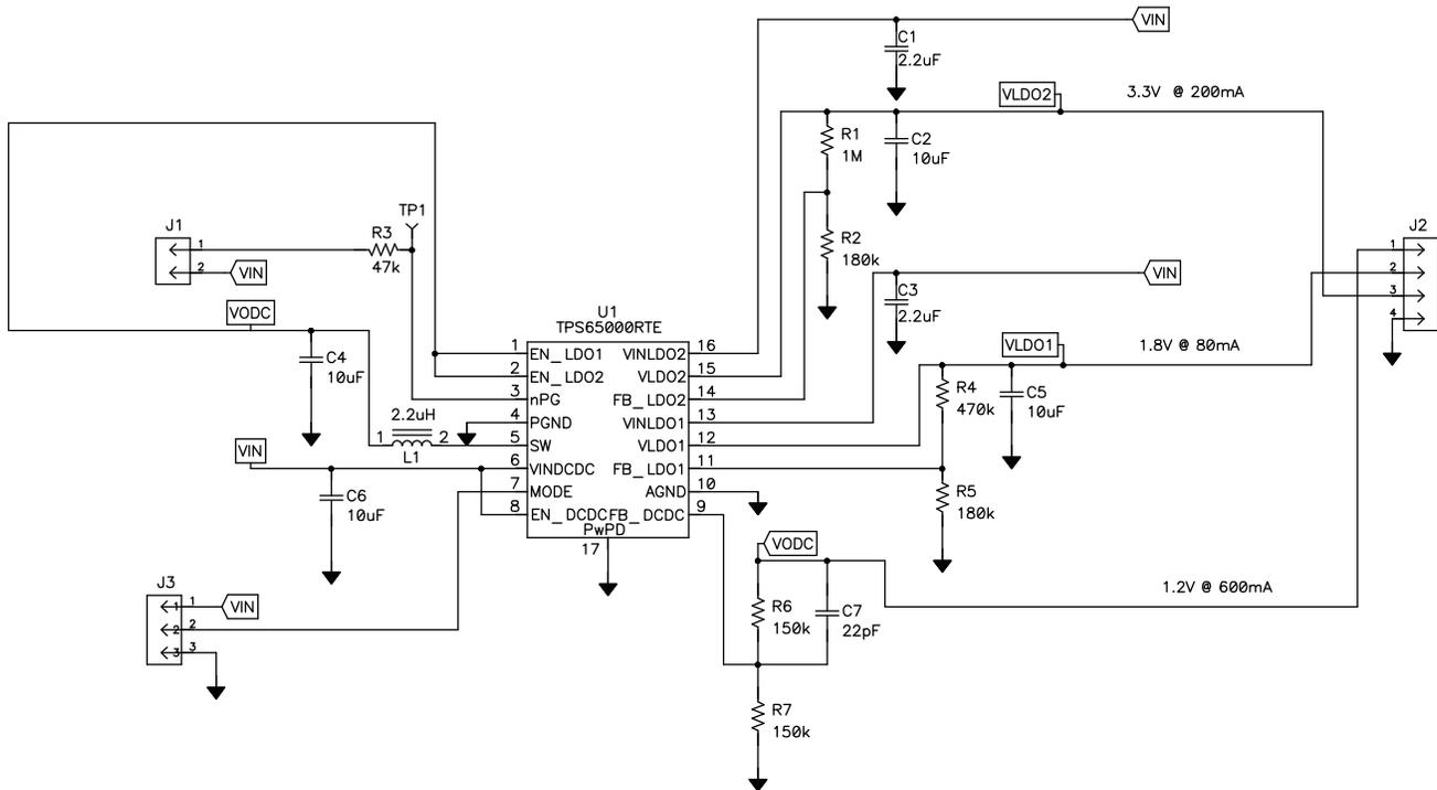
Figure 1. PMP5000 Reference Design Schematic
