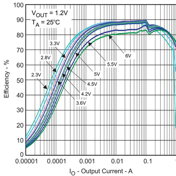
**Figure 3. Efficiency vs Output Current (TPS65000)**
