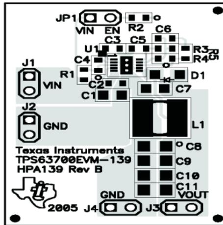
Figure 4. Inverter Improved Board Layout
