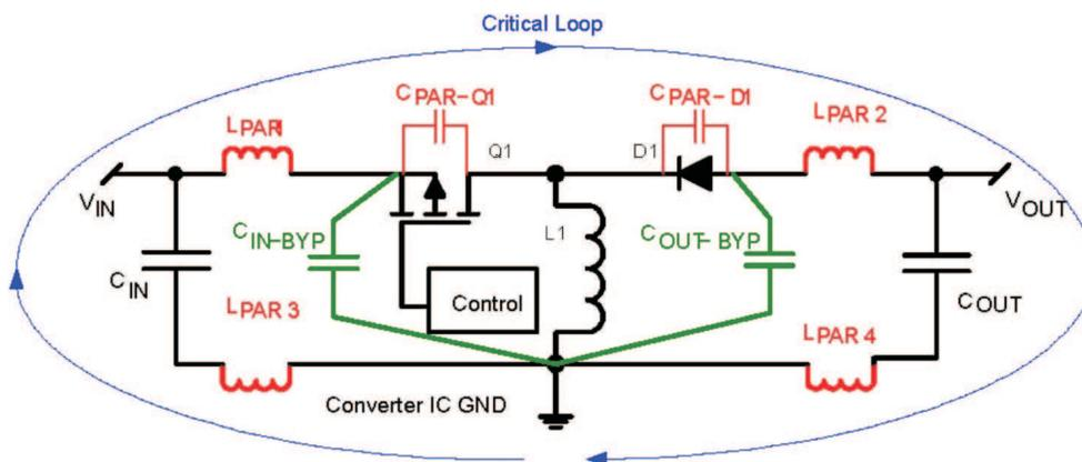
Figure 3. Buck-Boost (Inverting) Converter Schematic
