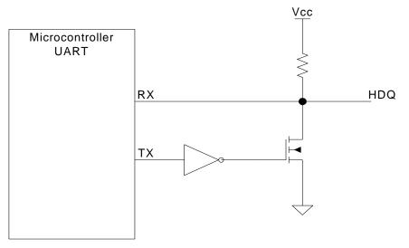
HDQ Comunication Circuit For UART Without Open Drain Outputs
