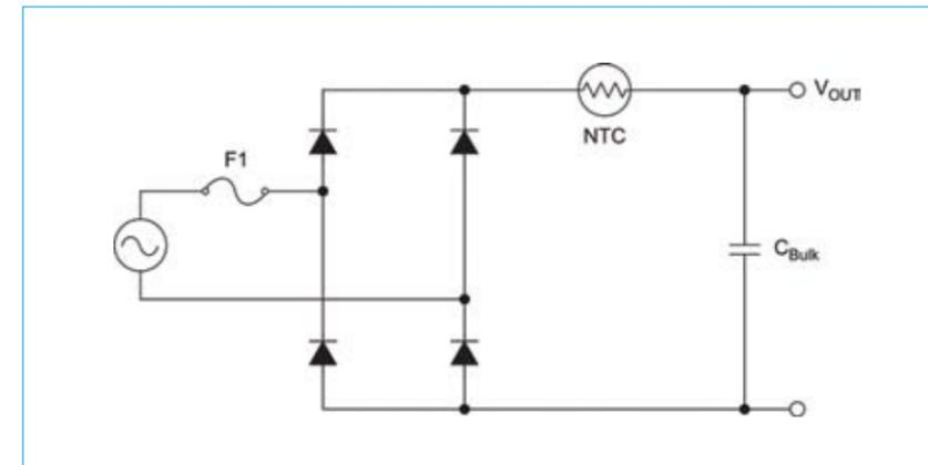
Figure 2: Typical inrush protection circuit.
