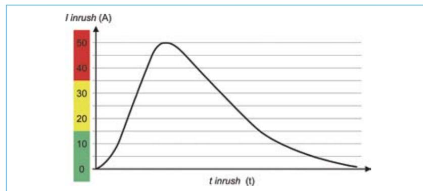
Figure 1: Typical 120VAC inrush current plot.
