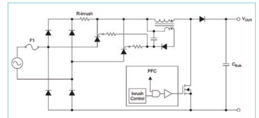
Figure 3: Inrush control function in PFC controller.
