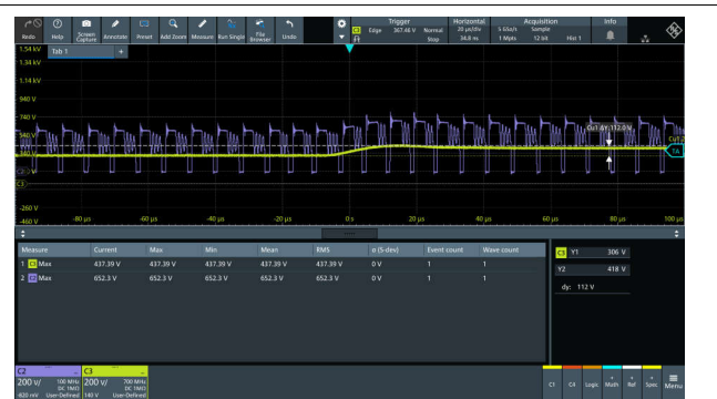
Figure 3-48. 1KV Surge at 230Vac input
