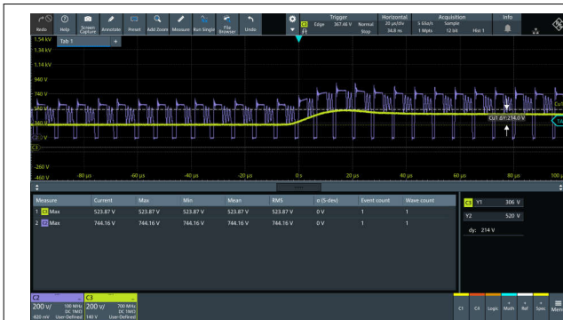
Figure 3-47. 2KV Surge at 230Vac input
