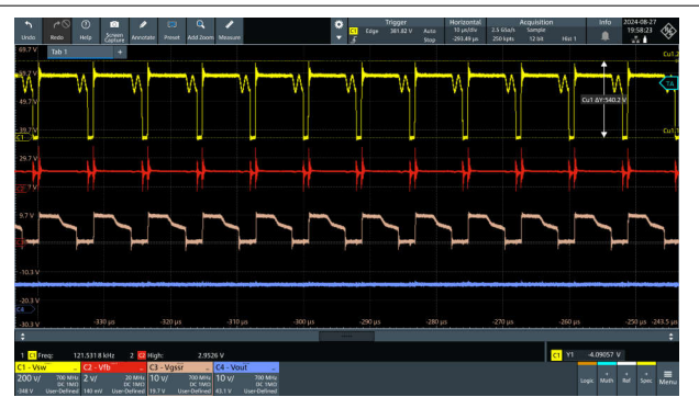
Figure 3-20. Vin = 264Vac, Vout = 9V
