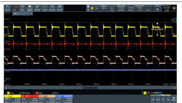
Figure 3-14. Vin = 115Vac, Vout = 15V
