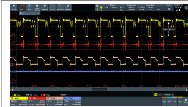
Figure 3-15. Vin = 230Vac, Vout = 15V
