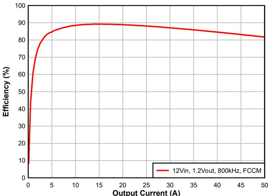
**Figure 4-1. Efficiency, V<sub>OUT</sub> Measured Using VO\_EFF, GND\_EFF, PVIN\_SNS, and PGND\_SNS Test Points**
