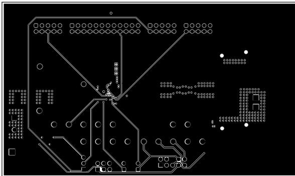
Figure 5-4. TPS546E25EVM-1PH Internal Layer 1 (Top View)
