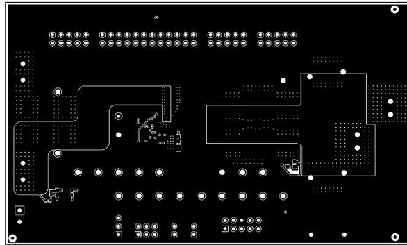
**Figure 5-8. TPS546E25EVM-1PH Bottom Copper Layer (Top View)**
