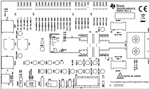
Figure 5-2. TPS546E25EVM-1PH Top Side Overlay View (Top View)
