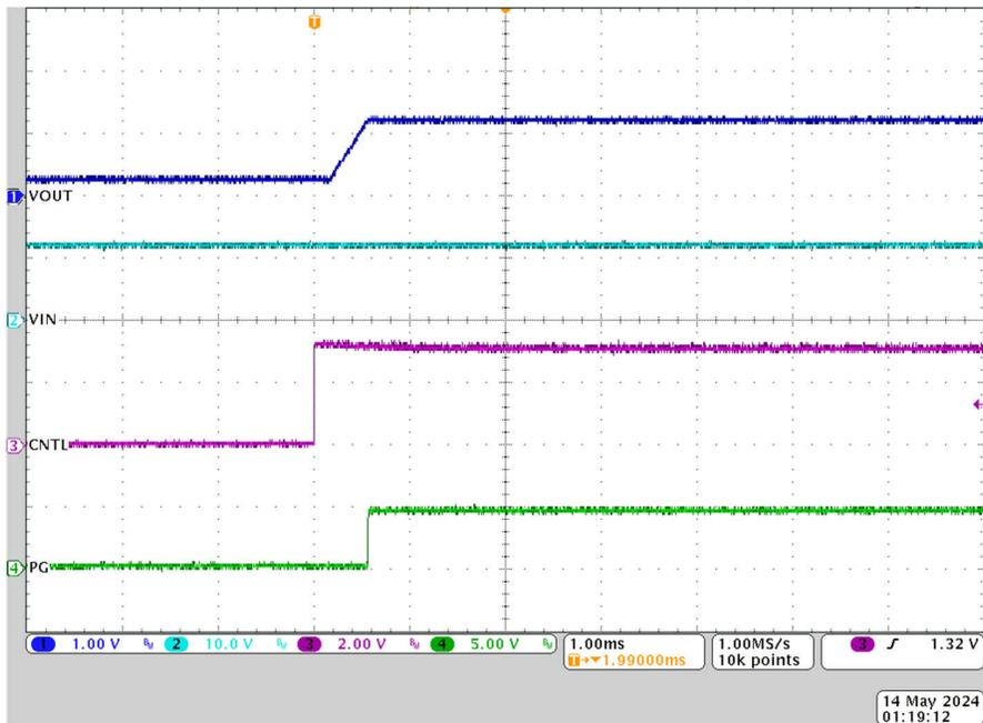
Figure 4-8. Start-Up From Control With Prebiased Output
