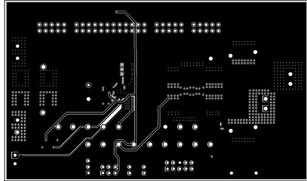
Figure 5-5. TPS546E25EVM-1PH Internal Layer 2 (Top View)
