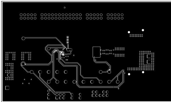
Figure 5-6. TPS546E25EVM-1PH Internal Layer 3 (Top View)
