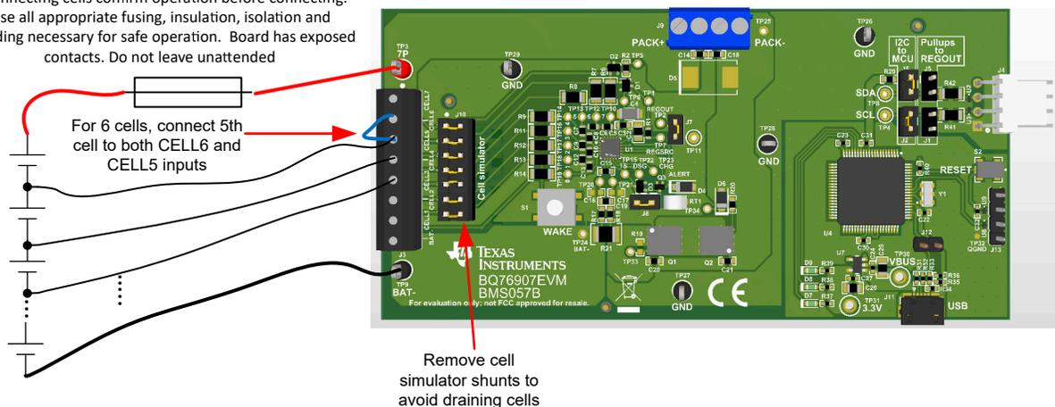
Figure 4-5. Example Connection with 6 Cells
