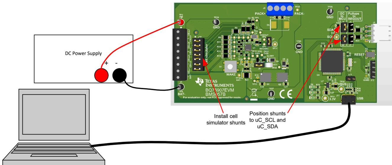
**Figure 2-1. EVM Connection for Basic Operation**
