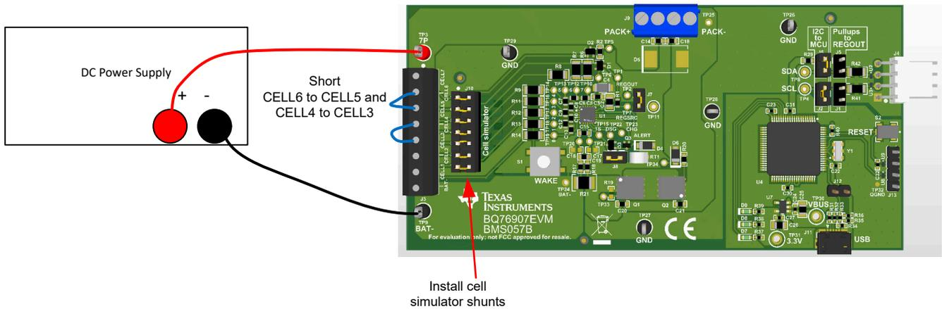
Figure 4-4. Example 5 Cell Simple Evaluation Configuration
