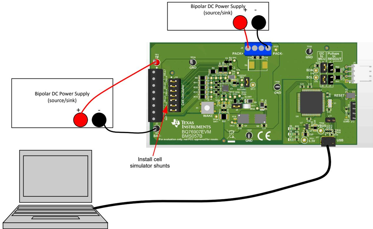
Figure 4-2. Evaluating with Charge or Discharge Current
