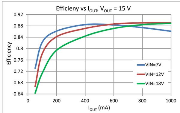
Figure 4-1. CV SEPIC Efficiency for  $V_{OUT} = 15 V$
