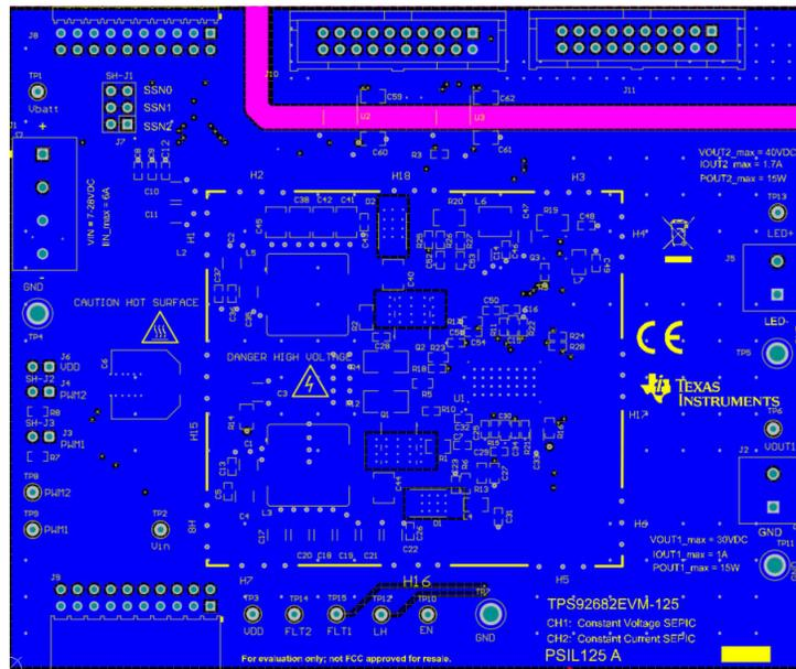
Figure 5-6. TPS92682EVM-125 Bottom Layer (Bottom View)
