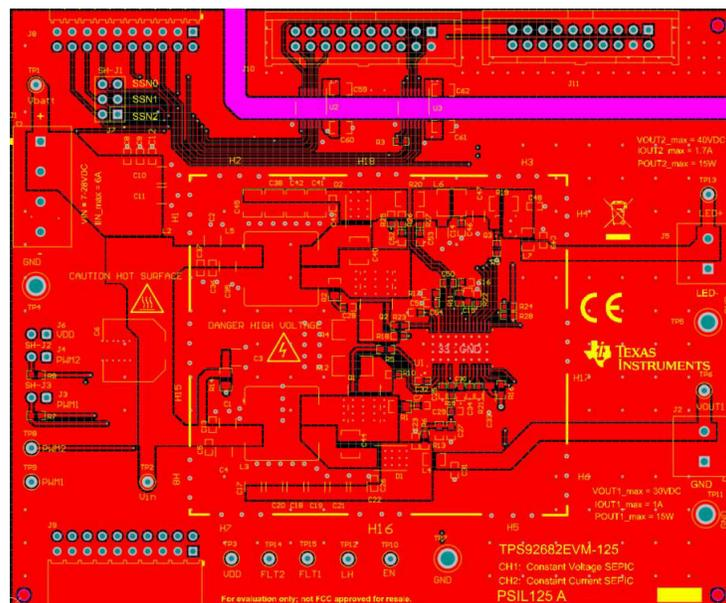
Figure 5-3. TPS92682EVM-125 Top Layer and Top Overlay (Top View)
