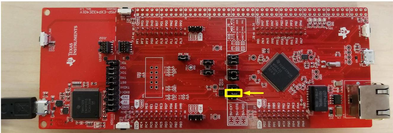
Figure 6-20. LaunchPad Connection for Programming
