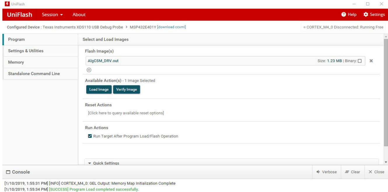
**Figure 6-25. UniFlash Programming, Step 5**
