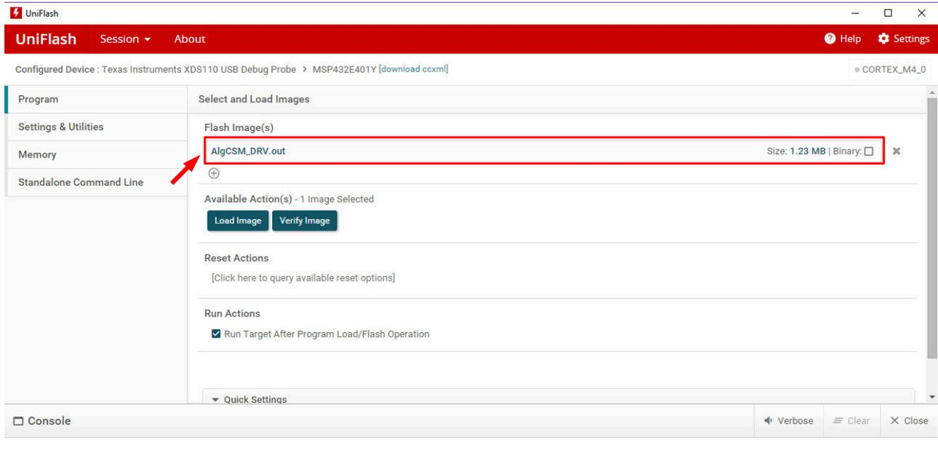
**Figure 6-23. UniFlash Programming, Step 3**
