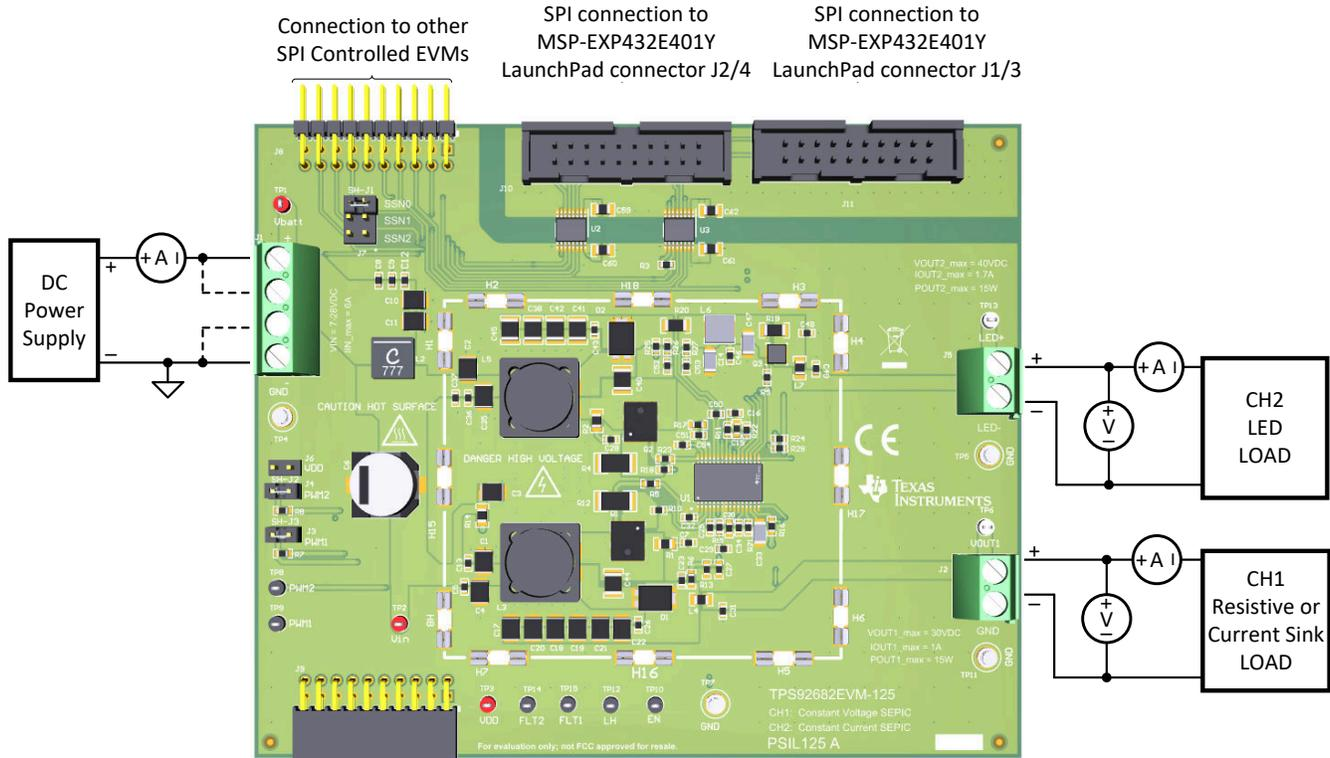
Figure 1-1. Component Connections
