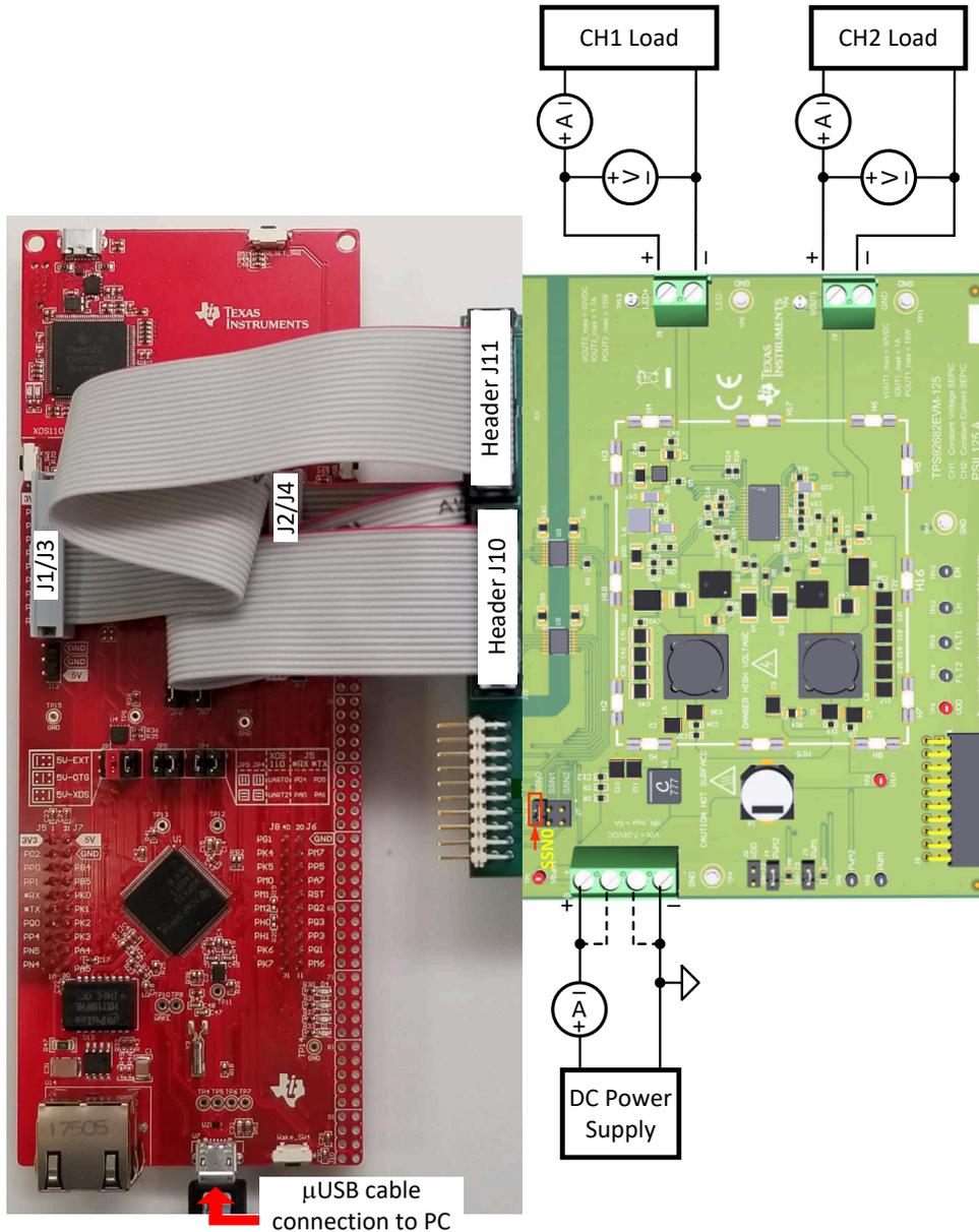
**Figure 7-1. LaunchPad Connection to TPS92682EVM-125**
