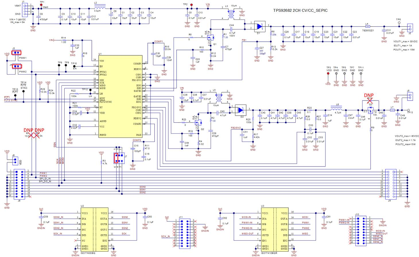
Figure 5-1. TPS92682EVM-125 Schematic
