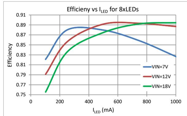
Figure 4-2. CC SEPIC Efficiency for  $V_{OUT} = 22 V$
