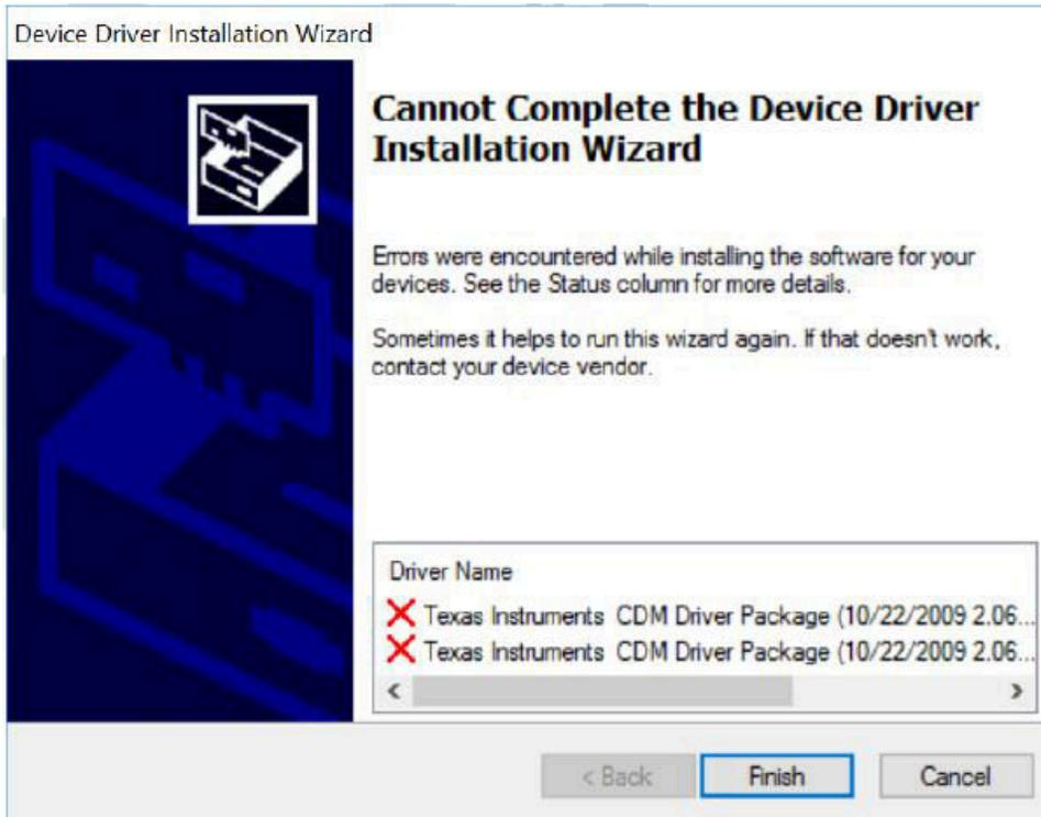
Figure 6-19. Driver Installation Error
