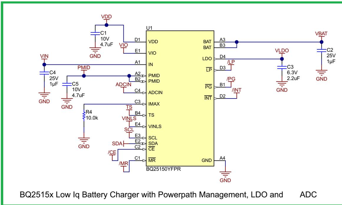
Figure 8. BQ25150 and Necessary Resistors and Capacitors
