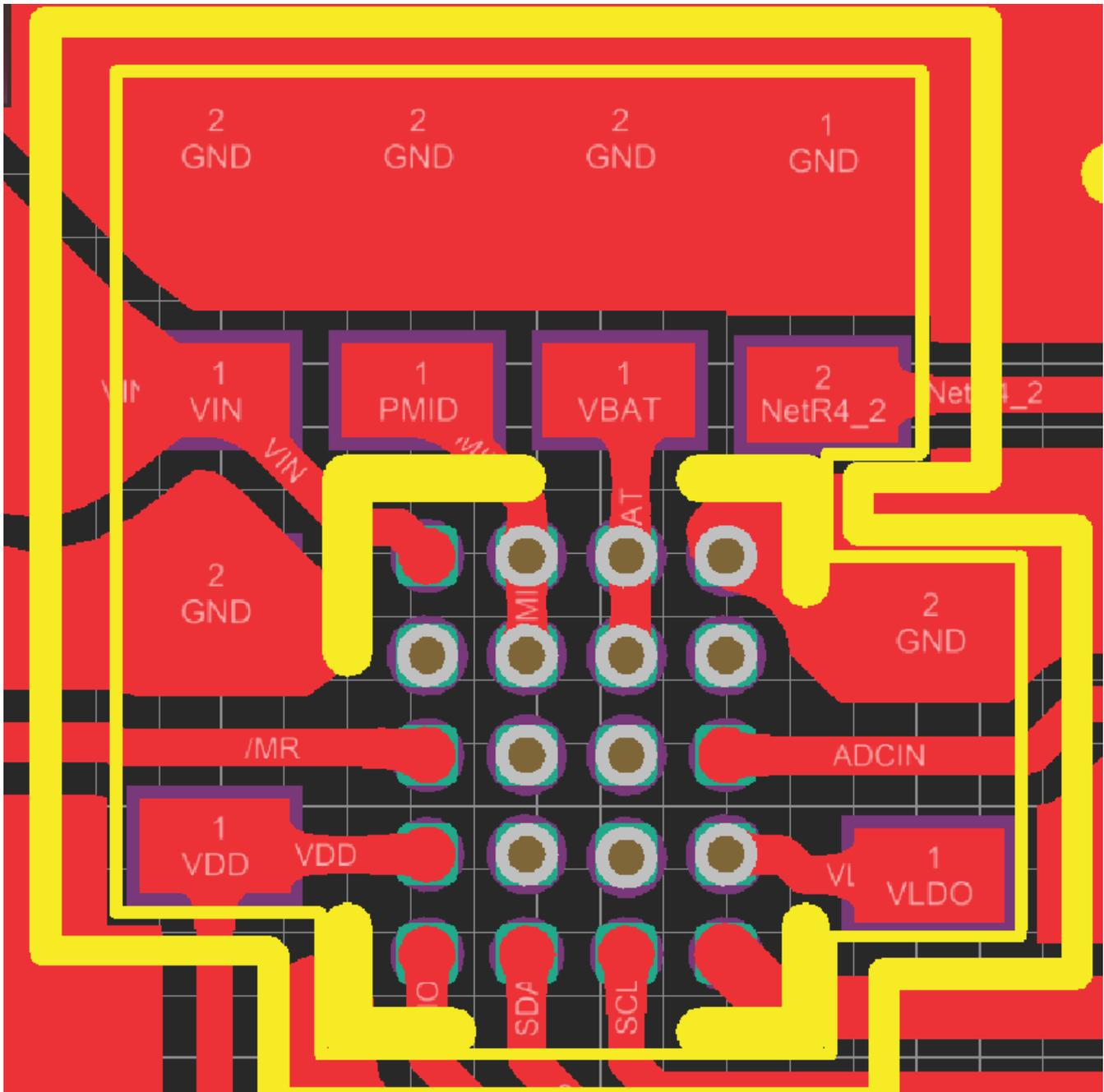
**Figure 3. 10 mil / 6 mil Vias on the Solder Ball Pads and 6 mil Traces Away From Pads and Vias**
