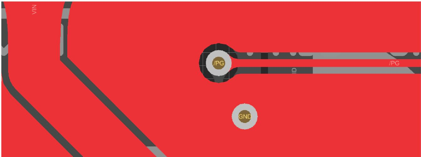
**Figure 4. 40-mil VIN Trace (Left) Significantly Larger Than 6 mil /PG Trace (Center Right) for Current Capacity**
