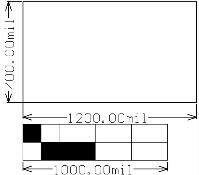
**Figure 17. Board Dimensions (Image is not Actual Size)**
