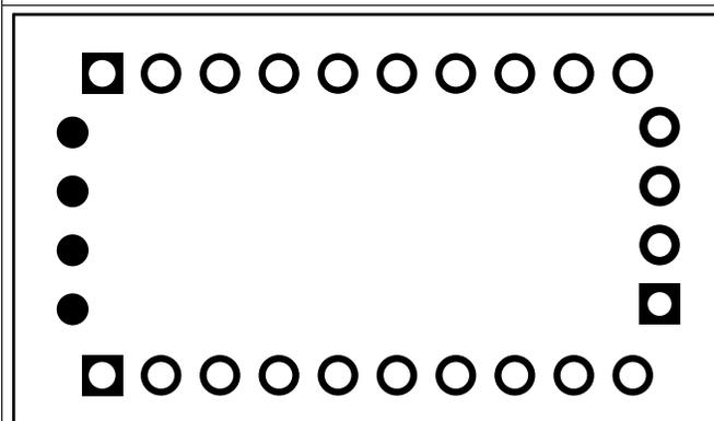
Figure 14. Bottom Solder Mask
