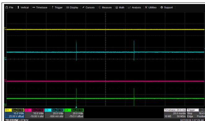
Figure 5.  $V_{IN} = 340 \text{ V}$ ,  $I_{OUT} = 0 \text{ A}$ , No Gate Drive Under Light Load (VG1, VG2)
