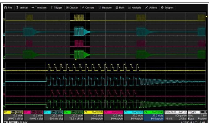
Figure 6.  $V_{IN} = 340 \text{ V}$ ,  $I_{OUT} = 0.3 \text{ A}$ , LLC is Operating In Burst Mode
