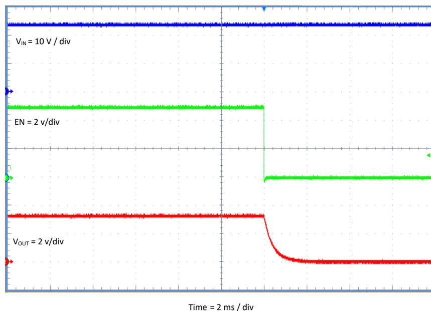
Figure 14. TPS54308EVM-876 Shutdown Relative to EN
