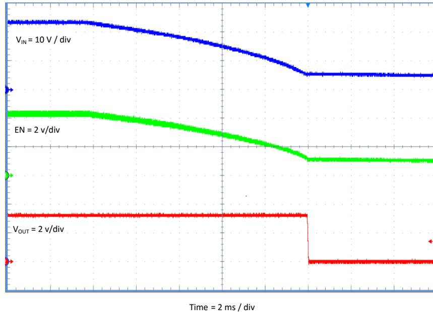
Figure 13. TPS54308EVM-876 Shutdown Relative to  $V_{IN}$
