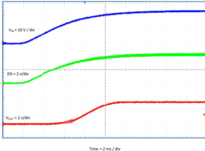
Figure 11. TPS54308EVM-876 Startup Relative to  $V_{IN}$
