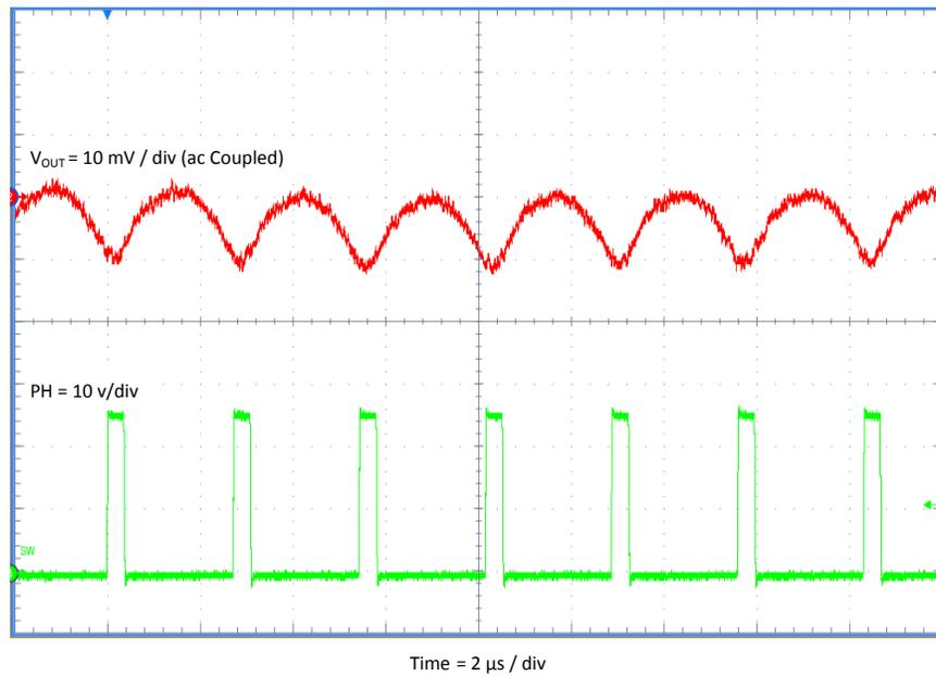
Figure 9. TPS54308EVM-876 Output Ripple, I<sub>OUT</sub> = 0 A
