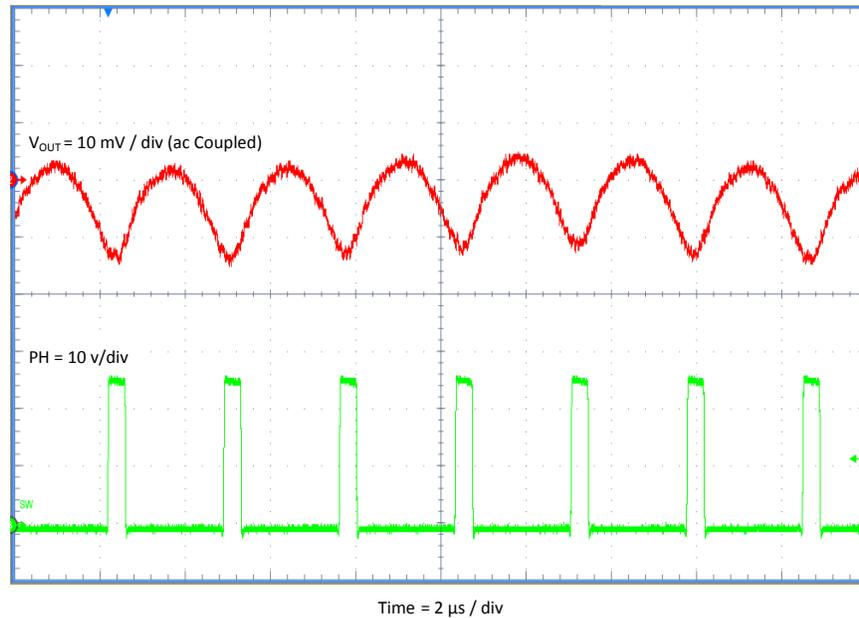
**Figure 6. TPS54308EVM-876 Output Ripple,  $I_{OUT} = 3\text{ A}$**
