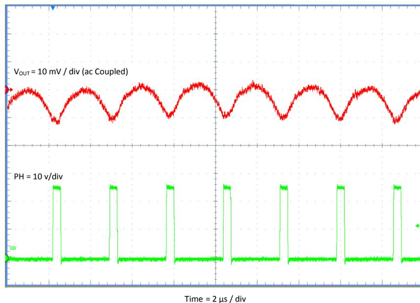
**Figure 7. TPS54308EVM-876 Output Ripple,  $I_{OUT} = 100\text{ mA}$**
