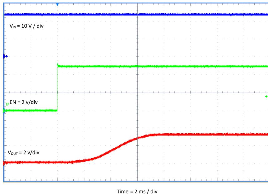
Figure 12. TPS54308EVM-876 Startup Relative to Enable
