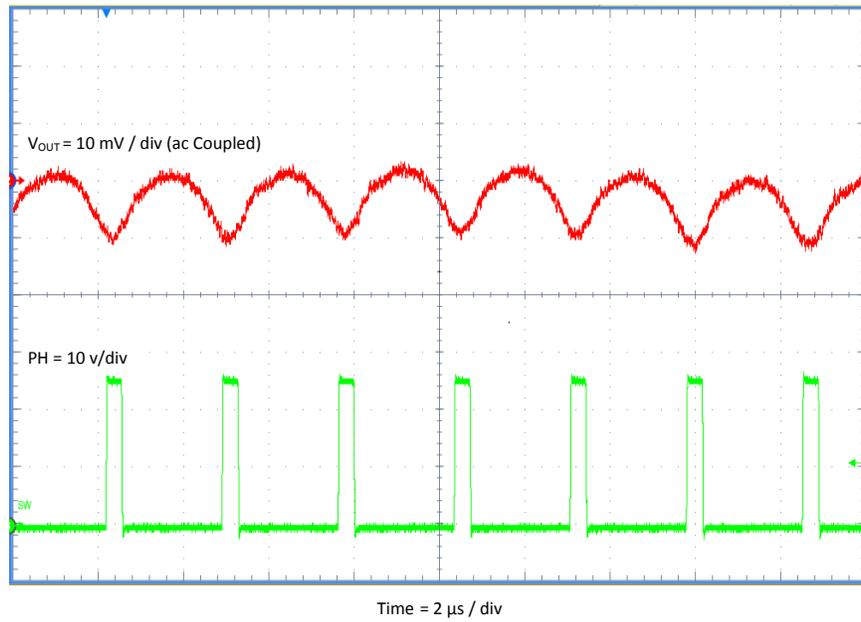
Figure 8. TPS54308EVM-876 Output Ripple, I<sub>OUT</sub> = 10 mA
