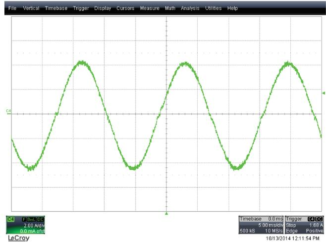
Figure 20. UCC29950EVM-631 Input Current (115-V<sub>AC</sub>, 60-Hz, full load 2 A/div.)
