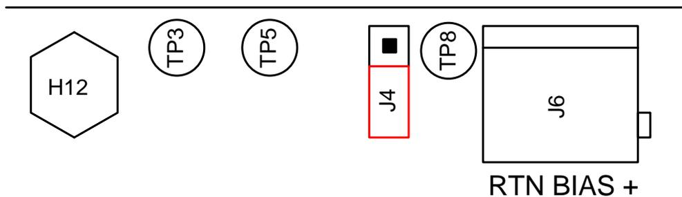
**Figure 5. J4 Link Setting for Self Bias Mode**
