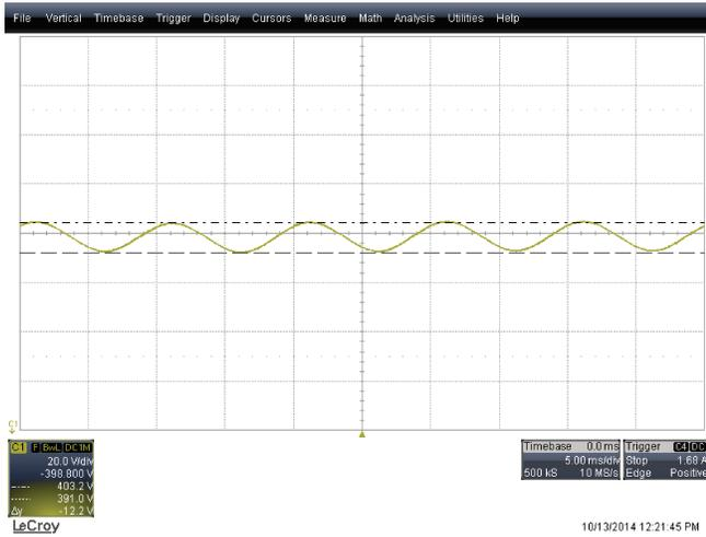
**Figure 22. UCC29950EVM-631 V<sub>BULK</sub> Voltage Ripple (115-V<sub>AC</sub>, 60-Hz input, full load)**
