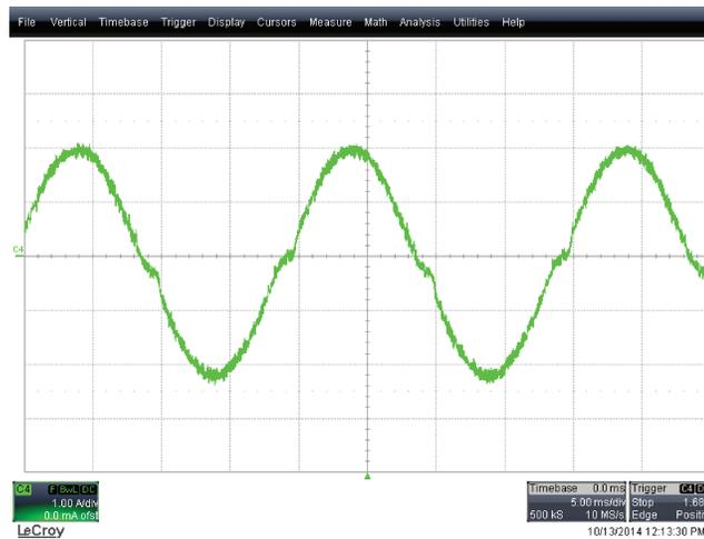
Figure 21. UCC29950EVM-631 Input Current (230-V<sub>AC</sub>, 50-Hz, full load 1 A/div.)
