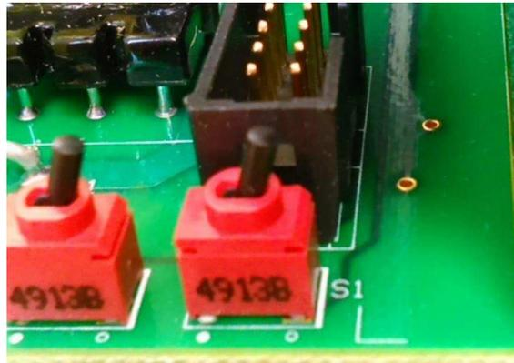
**Figure 6. S1 and S2 Settings for PFC and LLC Off
