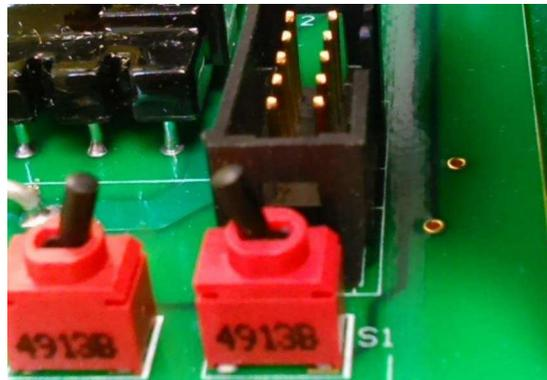
**Figure 8. S1 and S2 Settings for PFC Stage On, LLC Stage Off
