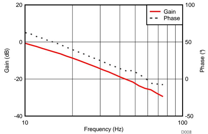
Figure 10. PFC Loop Gain/Phase at 300 W, 230 V
