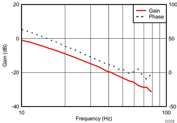
Figure 9. PFC Loop Gain/Phase at 300 W, 115 V
