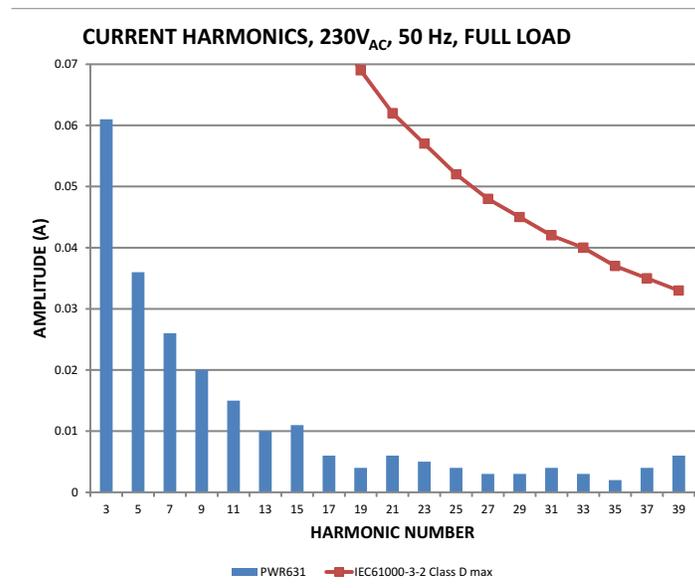
Figure 15. UCC29950EVM-631 Current Harmonics (230-V<sub>AC</sub>, 50-Hz input, full load)
