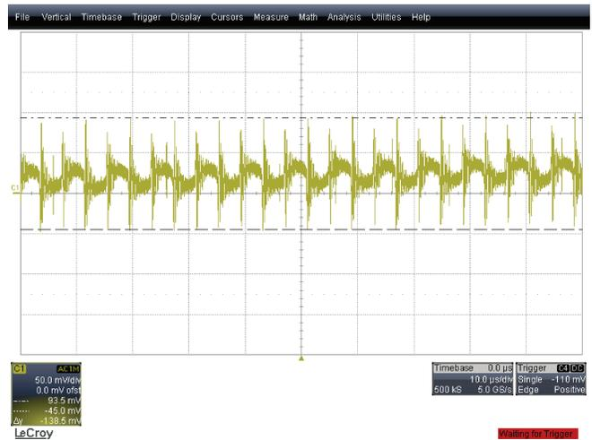
**Figure 25. UCC29950EVM-631 Output Noise (230-V<sub>AC</sub>, 50-Hz input, full load)**
