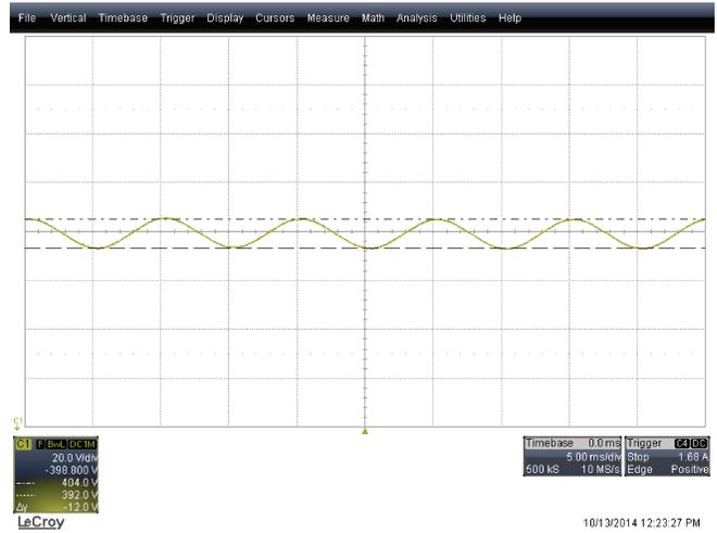
**Figure 23. UCC29950EVM-631 V<sub>BULK</sub> Voltage Ripple (230-V<sub>AC</sub>, 50-Hz input, full load)**
