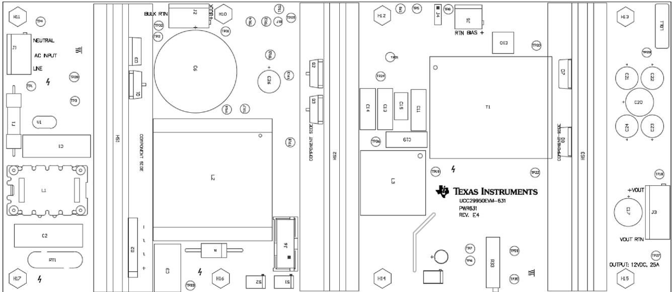
**Figure 34. UCC29950EVM-631 Top Layer Assembly Drawing (top view)**
