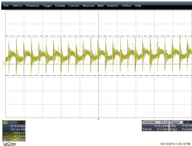
**Figure 24. UCC29950EVM-631 Output Noise (115-V<sub>AC</sub>, 60-Hz input, full load)**
