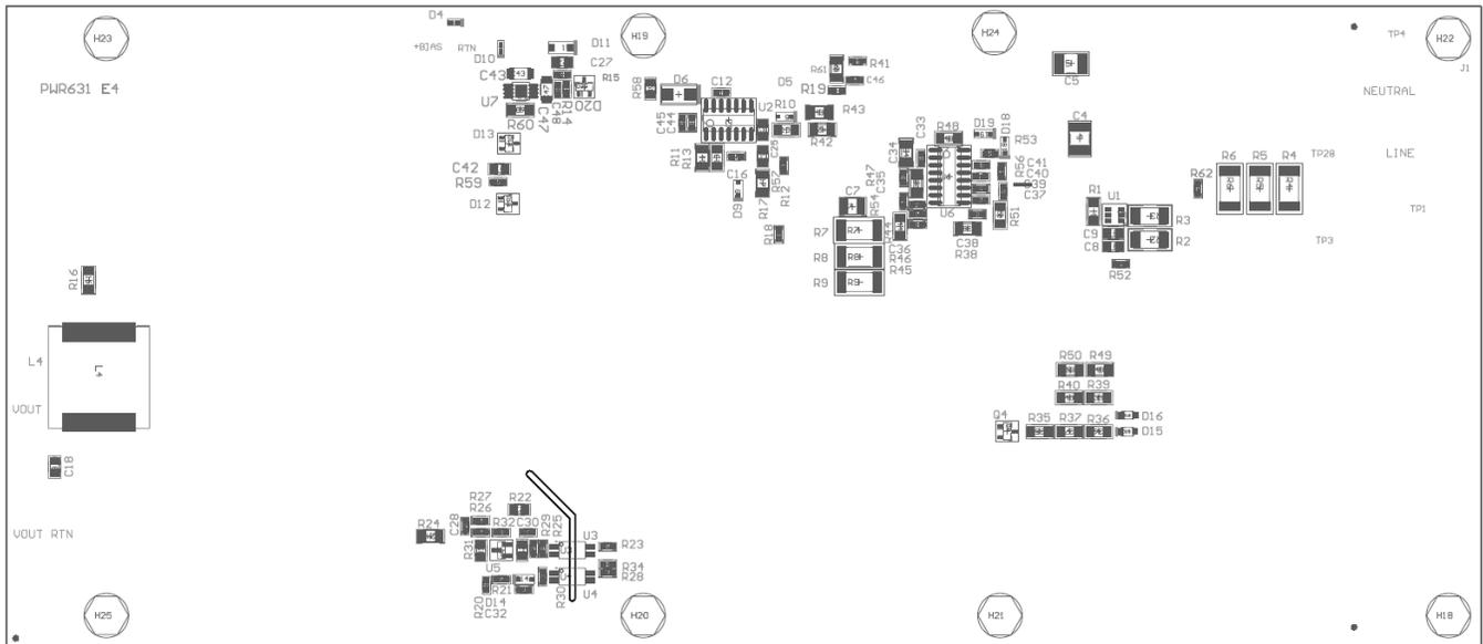
**Figure 35. UCC29950EVM-631 Bottom Layer Assembly Drawing (bottom view)**
