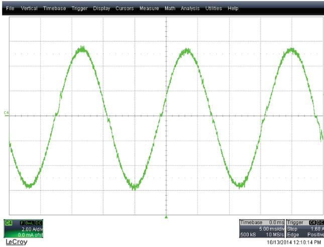
Figure 19. UCC29950EVM-631 Input current (90-V<sub>AC</sub>, 60-Hz, full load, 2 A/div.)
