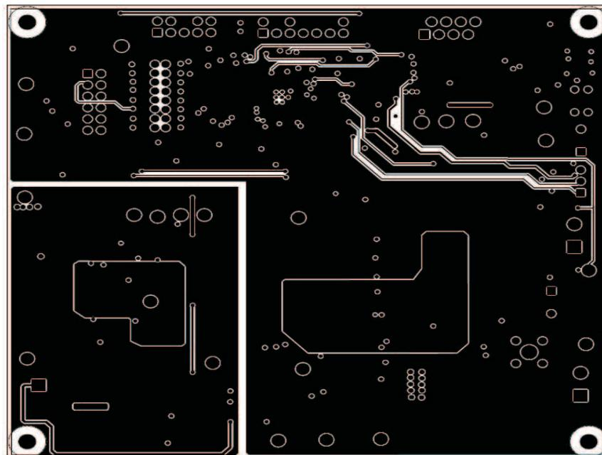
Figure 18. UCD3138HSFBEVM-029 Internal Layer 1 (top view)
