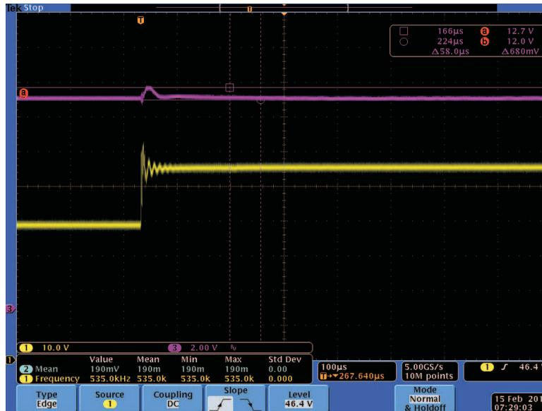
Figure 39.  $V_O$  Change from Digital Feed Forward Control
