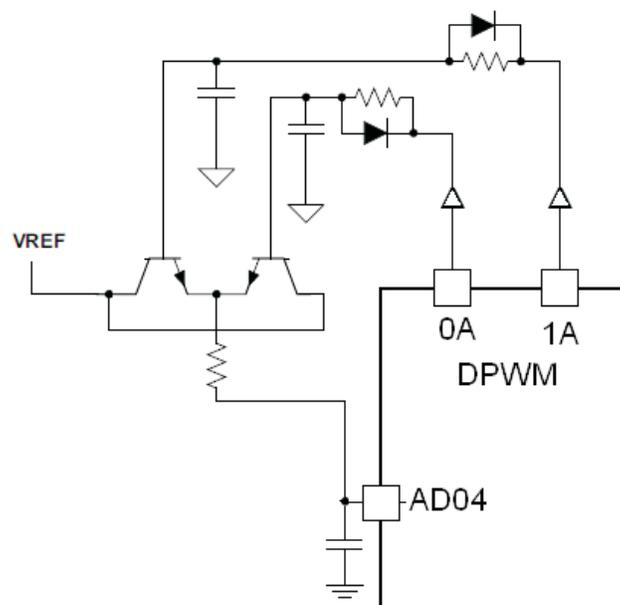
Figure 46. An Example of External Slope Compensation
