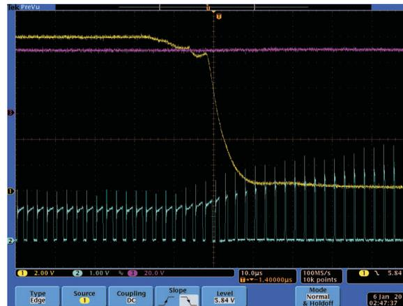
Figure 48. Short Circuit Protection Test
