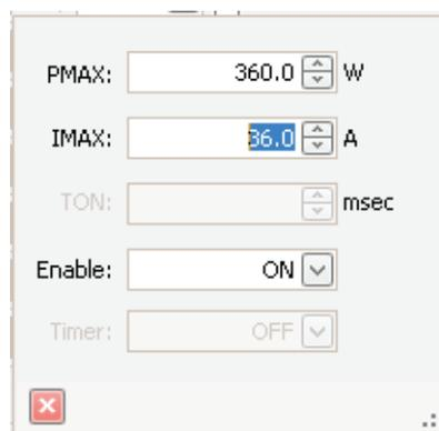
**Figure 44. CPCC Default Values and Adjustable through GUI**
