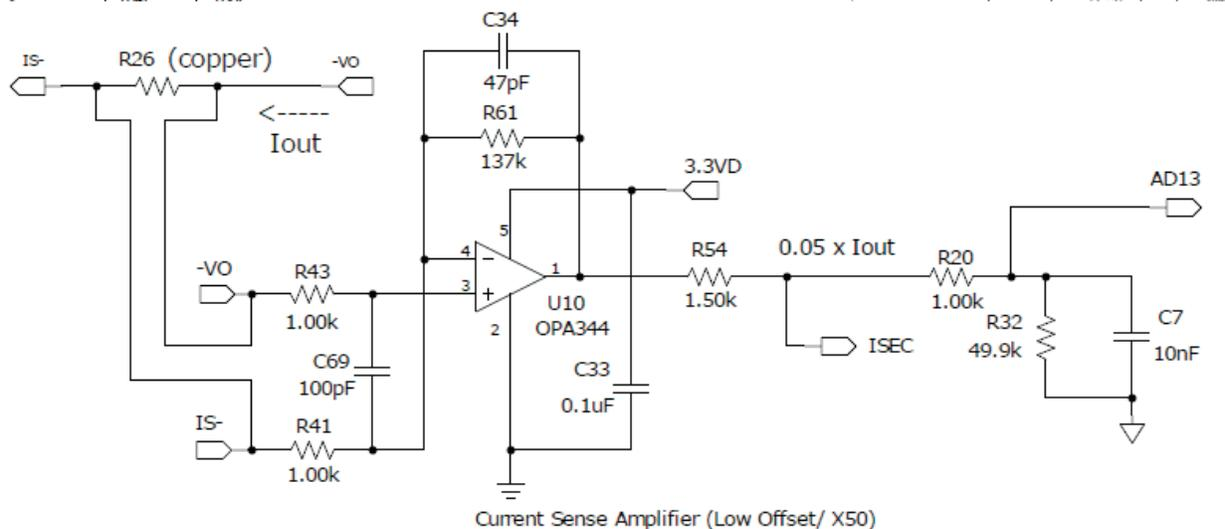
Figure 27. Load Current Sensing by PCB Copper
