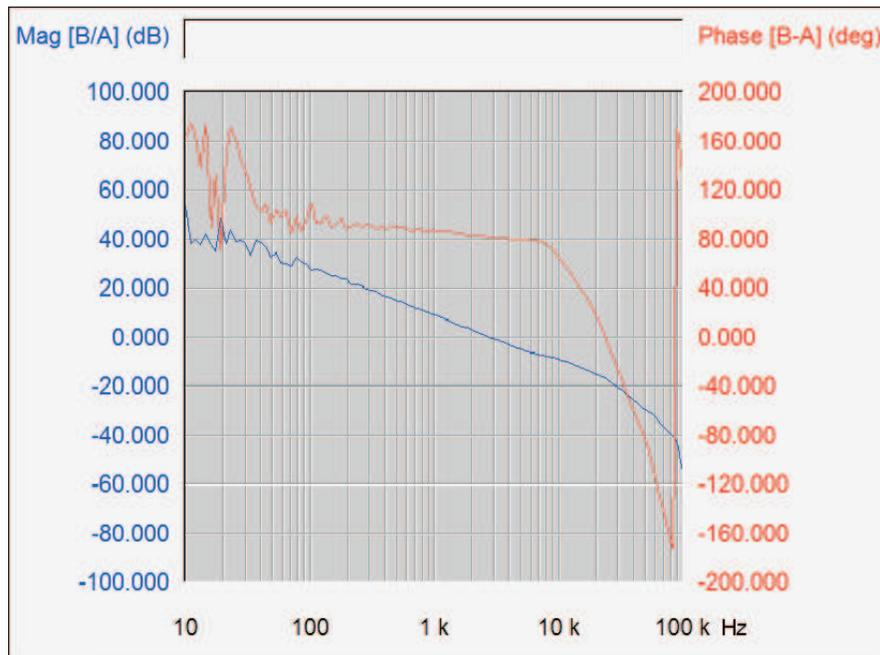
**Figure 13. Control Loop Bode Plots at 48 V<sub>DC</sub> and Half Load**
