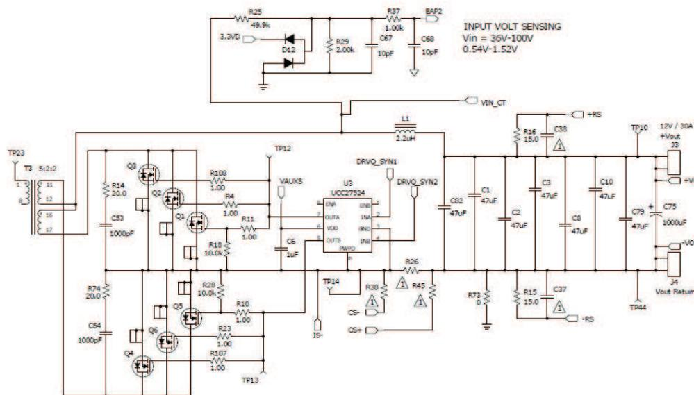
**Figure 26. Input Voltage Sensing Using Main Transformer**
