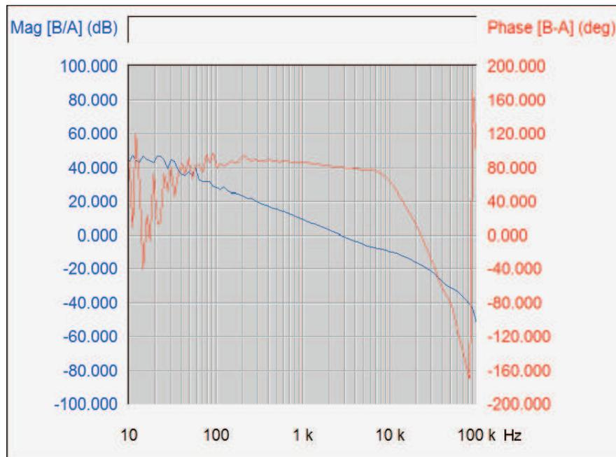
**Figure 14. Control Loop Bode Plots at 48 V<sub>DC</sub> and Full Load**
