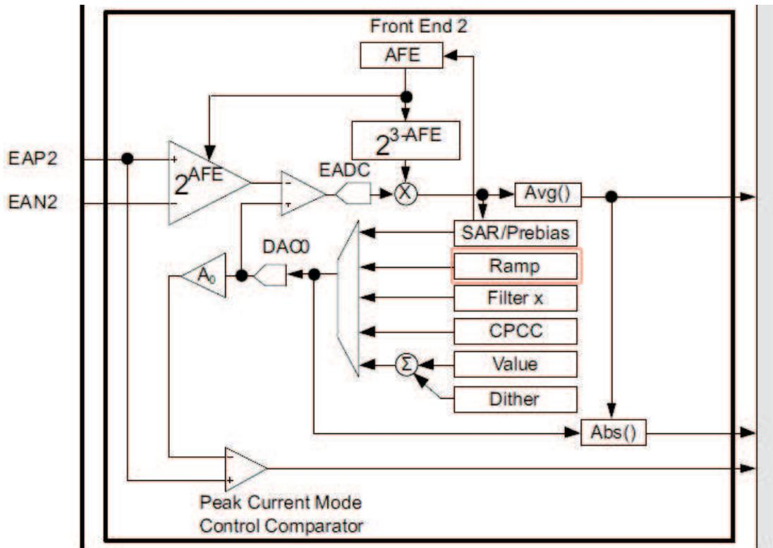
Figure 47. Peak Current Mode Control with Front End 2
