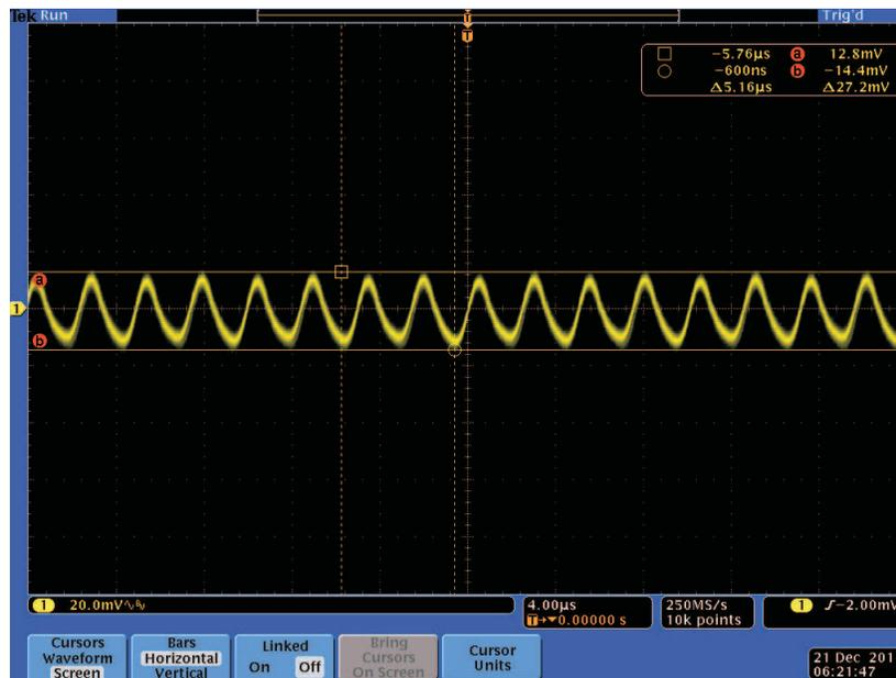
Figure 10. Output Voltage Ripple at 48 V<sub>DC</sub> and Half Load, 27.2 mV
