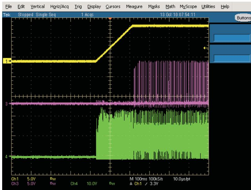
Figure 11. Output Turn On 48 V<sub>DC</sub> with Load Range (Ch 1 = V<sub>O</sub>, Ch 3 = DPWM1B, Ch 4 = V<sub>CT</sub>, Load = 1 A)
