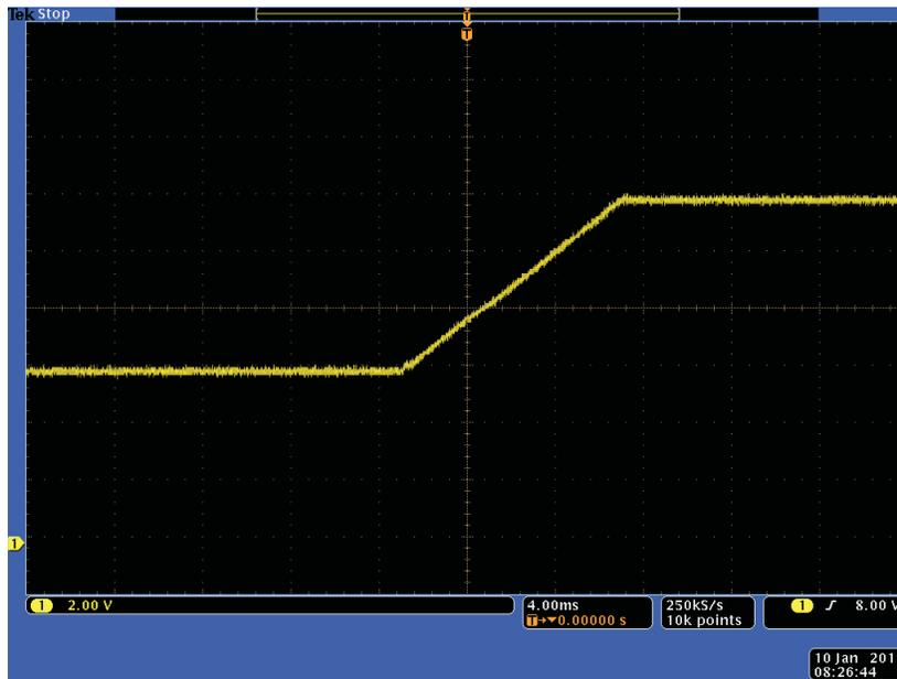
Figure 12. Output Turn On 48 V<sub>DC</sub> with 6-V Prebias
