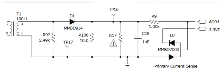
Figure 45. Cycle-by-Cycle Current Limit Sensing Circuit
