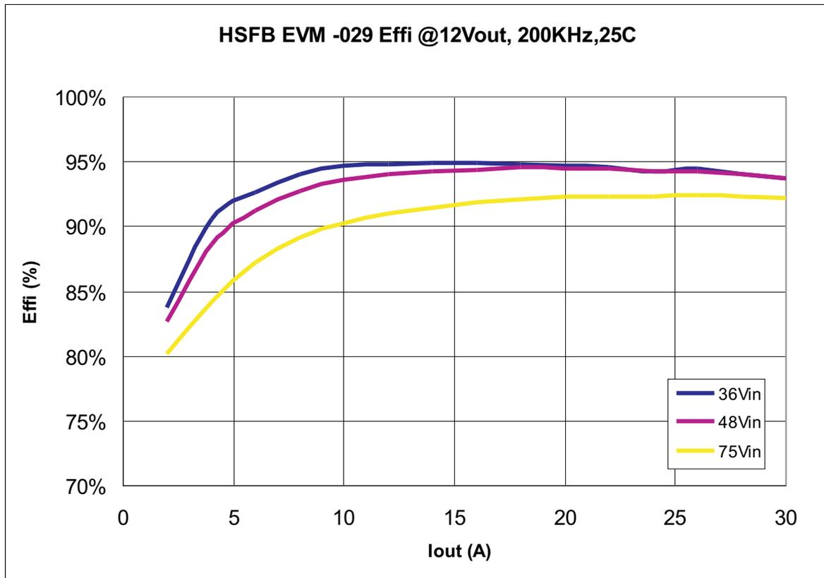
Figure 6. UCD3138HSFBEMV-029 Efficiency
