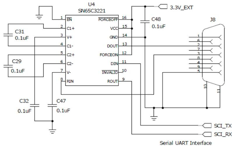
Figure 29. Serial Port Interface in the Converter
