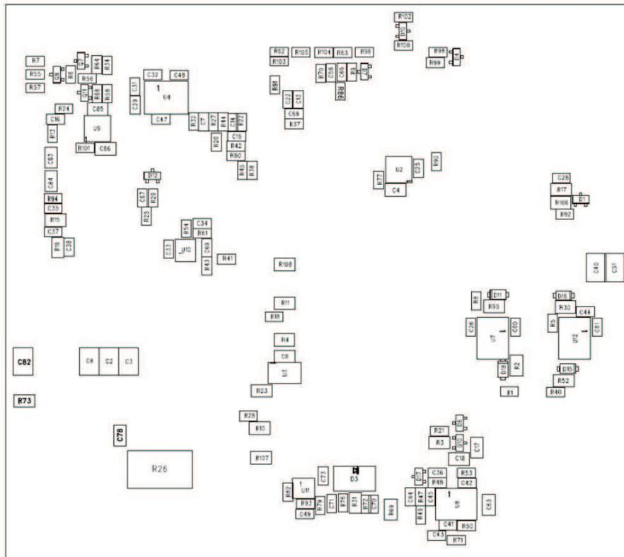
Figure 16. UCD3138HSFBEVM-029 Bottom Assembly Drawing (bottom view)
