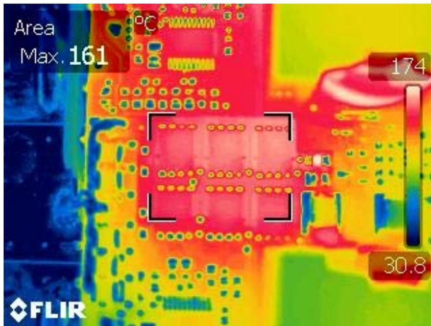
**5.4 Bottom Inductor Winding – No Airflow**
