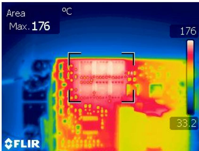
**5.7 Top Inductor Winding – No Airflow**
