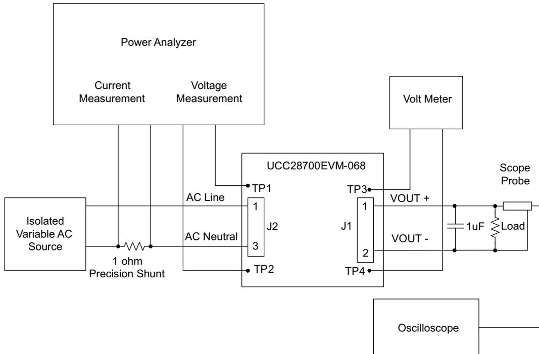
Figure 3. Test Setup
