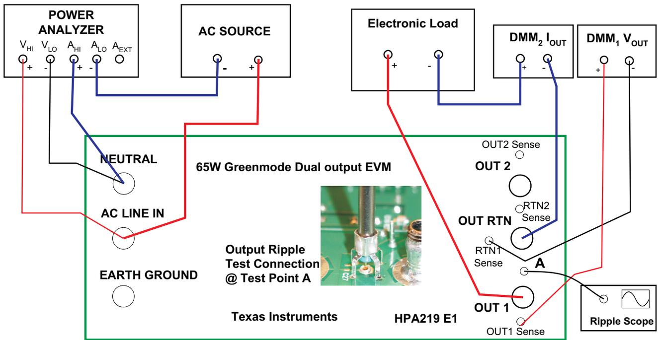
A Test point A may be found on the bottom side of the board.
