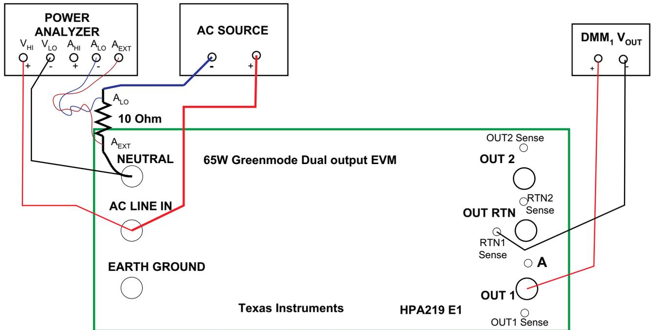
Figure 3. Test Setup for Standby Mode Operation.
