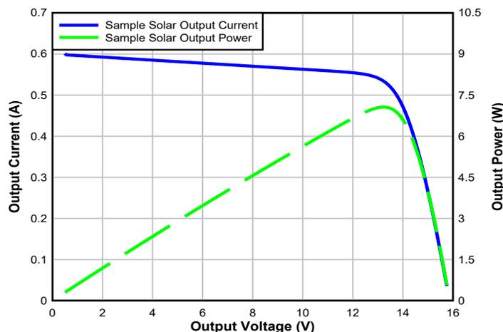
Figure 1-1. Sample I-V and P-V Curve
