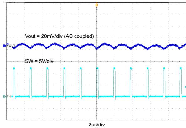
**Figure 5-6. Co-layout Board with TPS565201 Output Ripple,  $V_{IN} = 12\text{ V}$ ,  $V_{OUT} = 1.05\text{ V}$ ,  $I_{OUT} = 5\text{ A}$**
