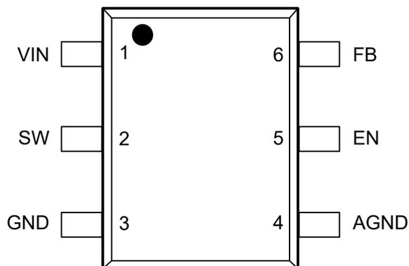
Figure 2-1. TPS56x242/7 Pin-out
