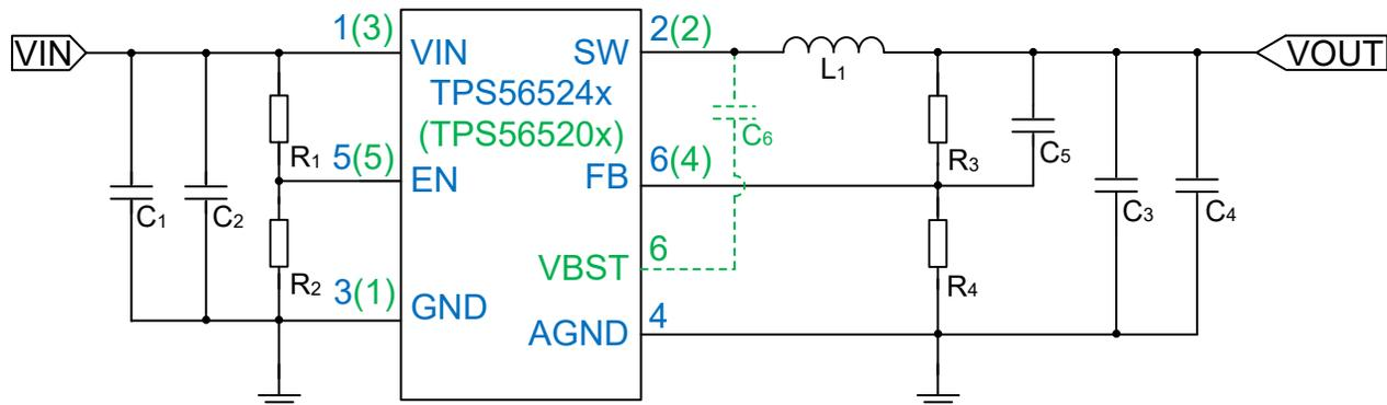
**Figure 3-1. Schematic Diagram to Achieve Co-lay**
