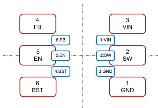
**Figure 4-1. Type 1 – Mirror Symmetrical Co-layout for TPS56x201/8 and TPS56x202/3/6/7**
