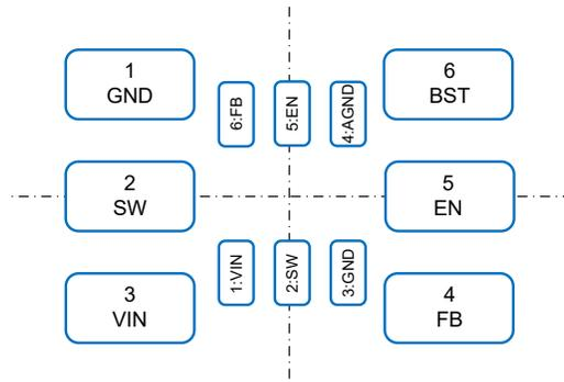
**Figure 4-2. Type 2 – Piggyback Co-layout for TPS56x201/8 and TPS56x242/7**
