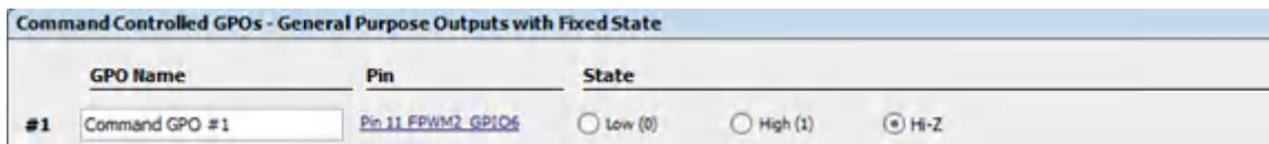
Figure 4-1. Configure GPIO to Hi-Z
