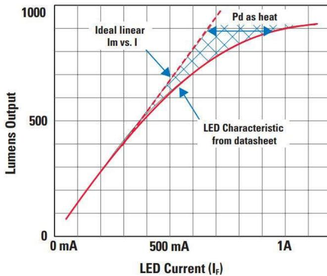
**Figure 5-1. Lumens Output Versus LED Current**
