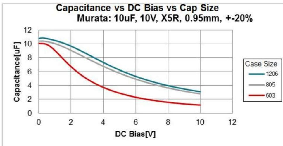
Figure 4-2. Capacitance Versus DC Bias
