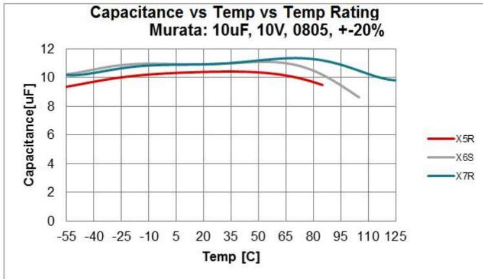
Figure 4-1. Capacitance Versus Temperature
