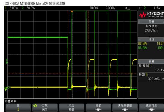
Figure 2-4. Switching Frequency During the Dimming off
