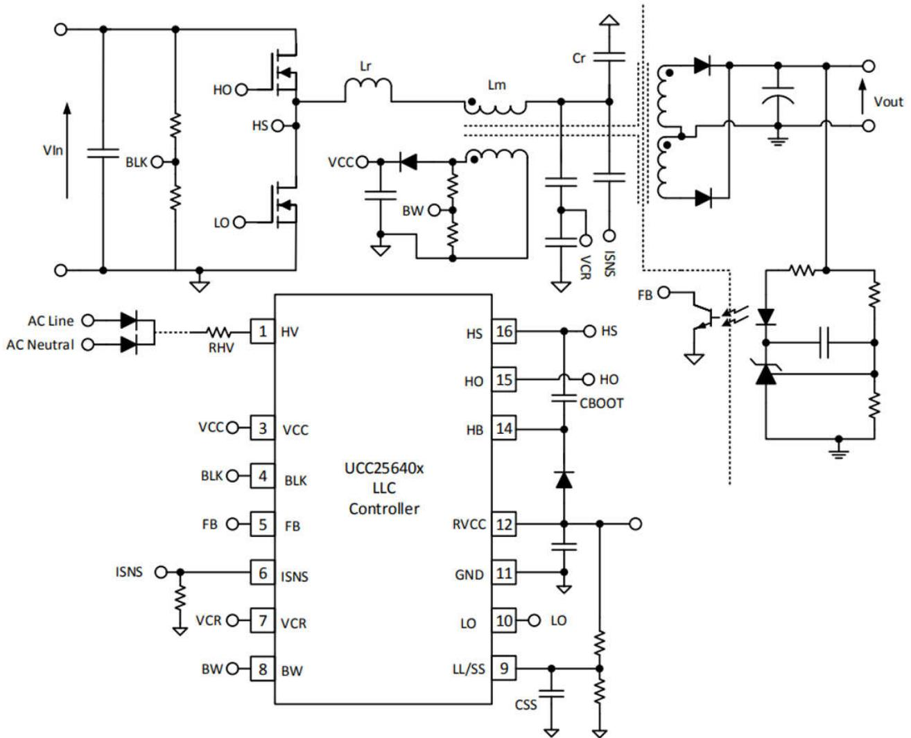
Figure 1-1. UCC25640X Simplified Schematic
