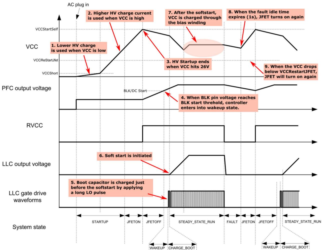
Figure 3-1. Timing Diagram of System State Machine for UCC256402 and UCC256404
