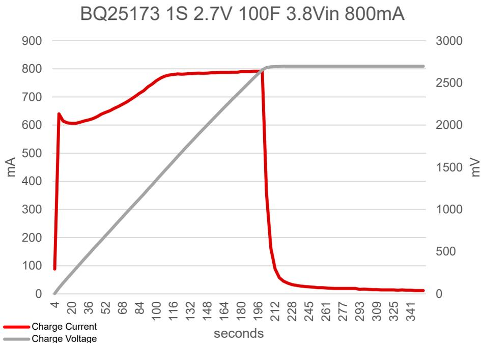
**Figure 8-1. Super Capacitor Charge Profile**
