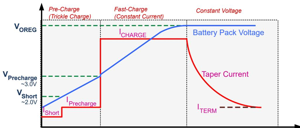
Figure 2-1. Typical Li-Ion Battery Charging Profile CC-CV
