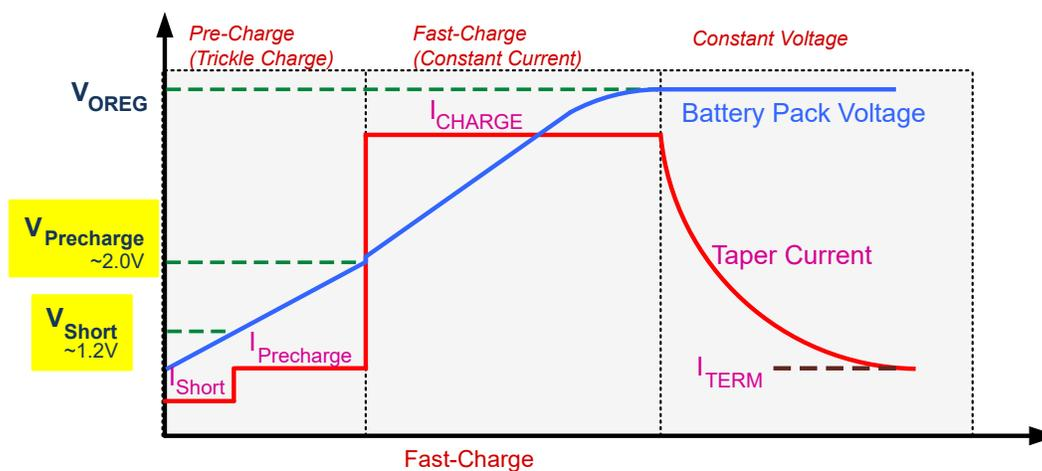
Figure 4-1. LiFePO4 Charge Profile
