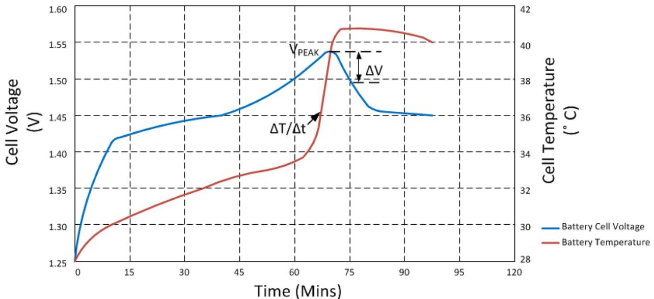
Figure 6-1. NiMH Fast Charge Profile
