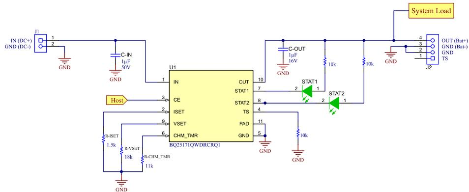
Figure 4-1. NiMH 200-mA Time Charge Design
