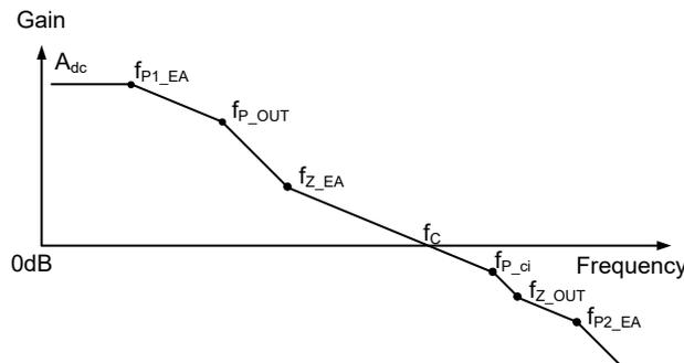
**Figure 2-1. Bode Plot of PCM Buck Converter Open Loop Response**
