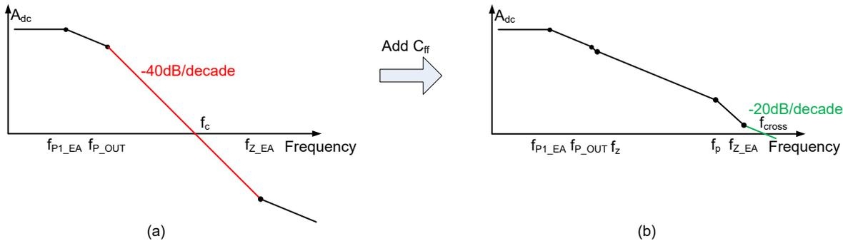
Figure 4-2. Correct Method to use  $C_{ff}$  by Adding Both the  $C_{ff}$  Zero and Pole Inside Bandwidth
