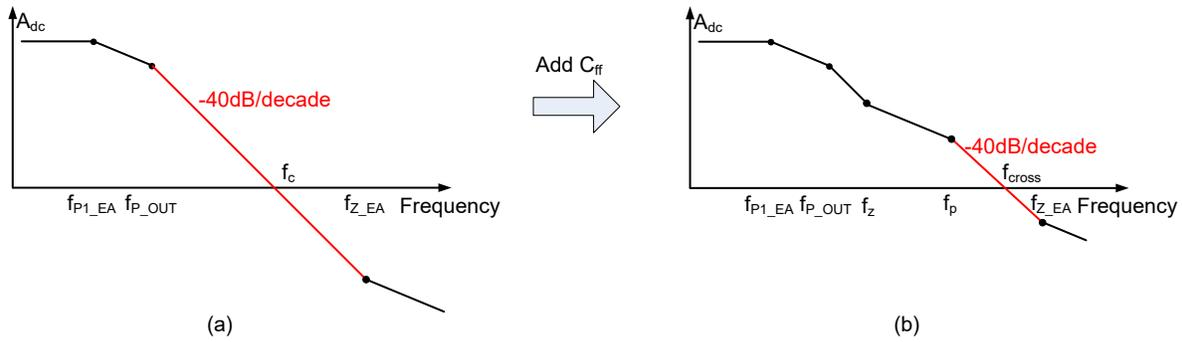
**Figure 4-3. Incorrect Method to use  $C_{ff}$  by Adding Both the  $C_{ff}$  Zero and Pole Inside Bandwidth**
