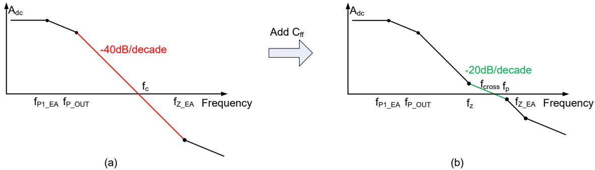
Figure 4-1. Correct Method to use  $C_{ff}$  by Only Adding  $C_{ff}$  Zero Inside Bandwidth
