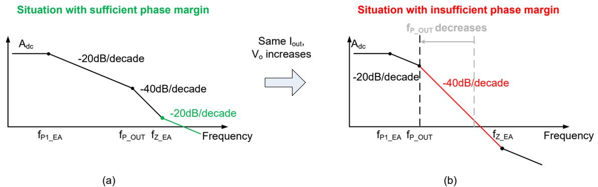
**Figure 2-3. Loop Gain of TPS62933 With Constant Output Current  $I_{out}$  (a) Low  $V_O$  With  $-20$  dB/dec Crossing (b) High  $V_O$  With  $-40$  dB/dec Crossing**
