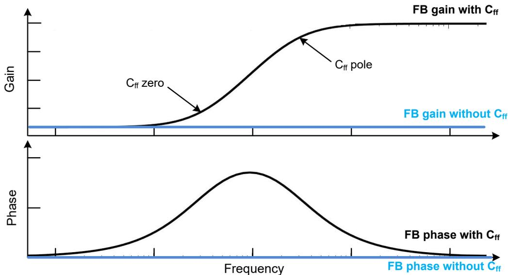
Figure 3-2. Bode Plot of Feedback Divider Transfer Function Including  $C_{ff}$
