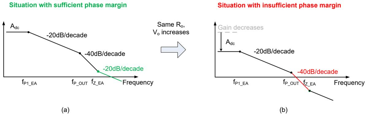
**Figure 2-2. Loop Gain of TPS62933 With Fixed Load Resistance  $R_O$  (a) Low  $V_O$  With  $-20$  dB/dec Crossing (b) High  $V_O$  With  $-40$  dB/dec Crossing**
