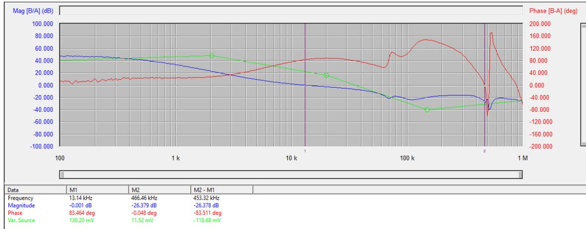
Figure 5-1. Bode Plot With the Selected Feedforward Capacitor
