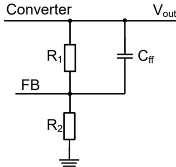
Figure 3-1. Scheme of Feedback Divider Including Feedforward Capacitor
