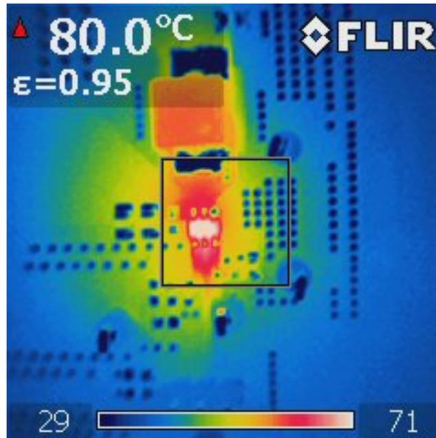
**Figure 5-2. Thermal Scan of TPS56339 EVM**
