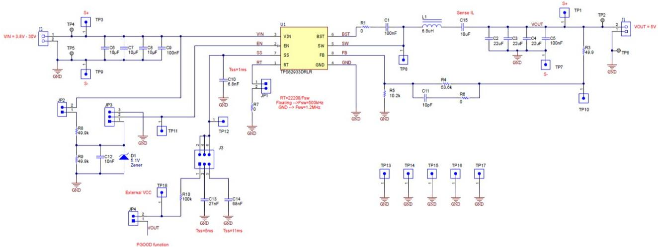
Figure 4-1. Typical Application Circuit of TPS62933 Device
