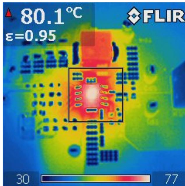
**Figure 5-3. Thermal scan of TPS54335A EVM.**
