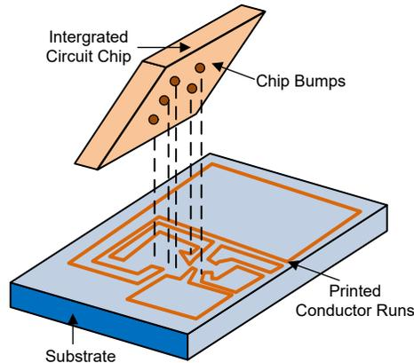
**Figure 3-1. Simplified Structure of Flip Chip on Lead Package**
