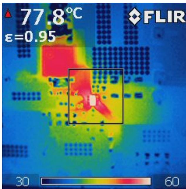
**Figure 5-1. Thermal Scan of TPS62933 EVB**
