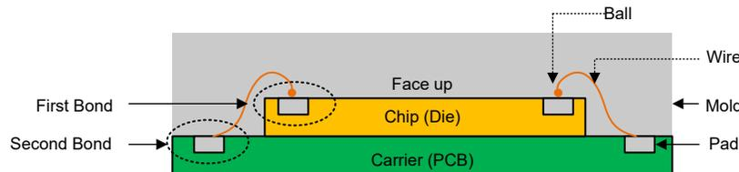
**Figure 2-1. Simplified Structure of Bonding Wire Package.**
