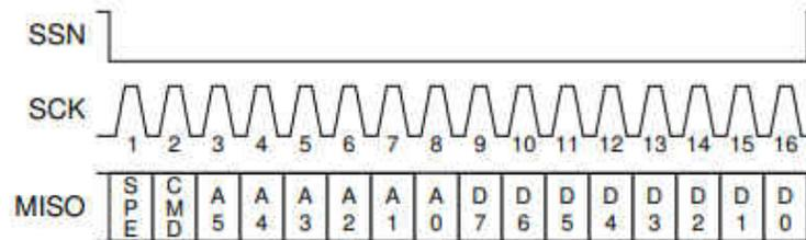
**Figure 7-25. Write Response Frame Format**
