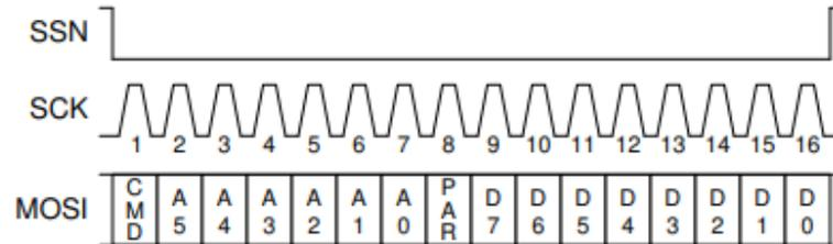
Figure 7-23. Command Frame Format
