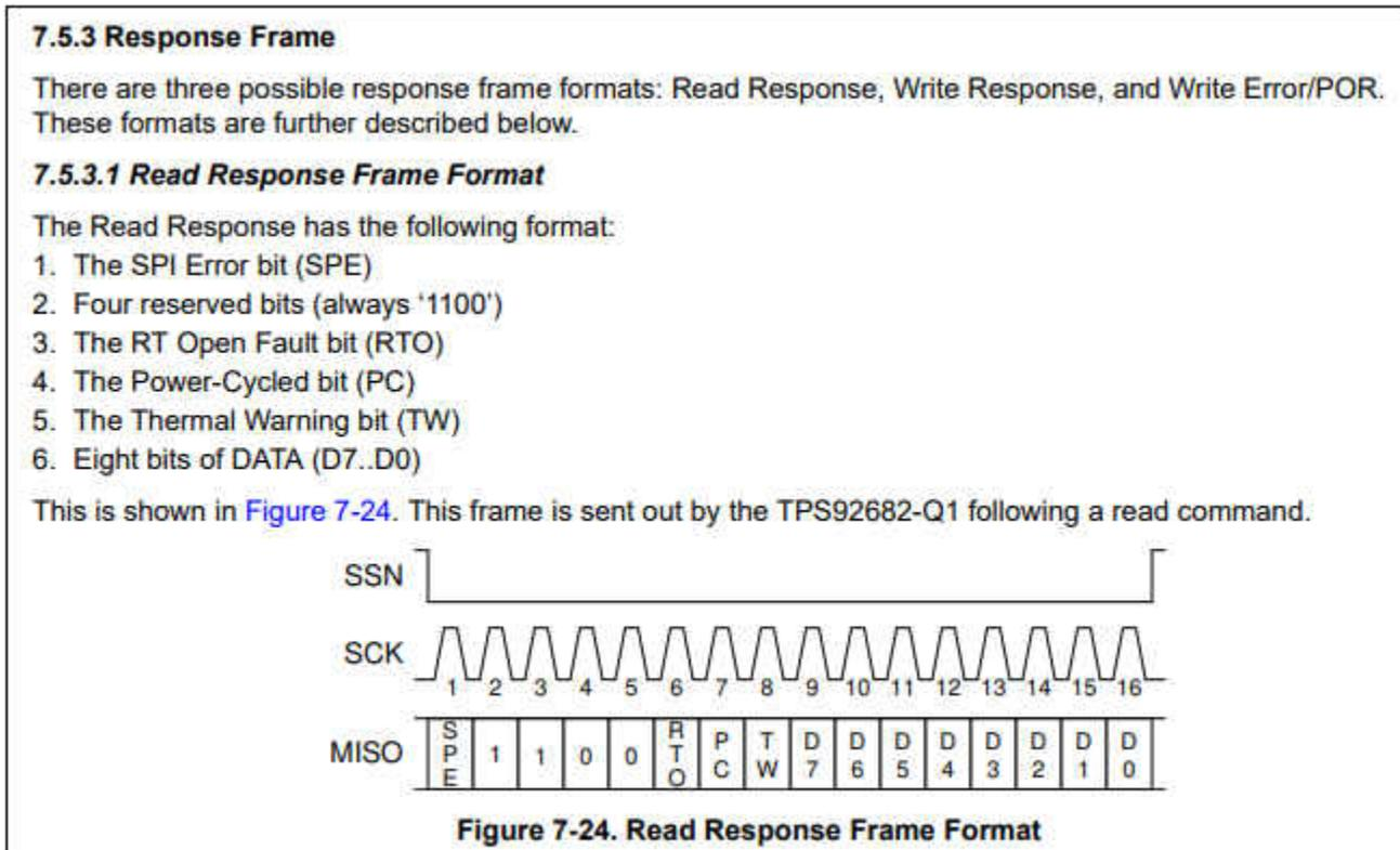
The command frame ([Build a Frame](#)) is SPI MOSI and the response is found in SPI MISO following it. The SPI MOSI command issued = 0x23 0x00. In this example the return (MISO result of 2 reads per SPI) has a status byte of 0x60 with a data byte of 0x02 indicating: CH2UV: Output undervoltage fault (CH2UV is disabled if 2PH is set to '1'). For a detailed explanation of the expected SPI bus return value with the TPS92682-Q1, visit the [TI E2E™ support forum](#).
