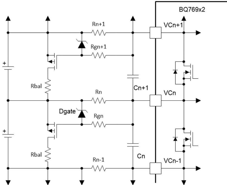
Figure 2-4. Balancing Circuit Using External P-Channel FETs
