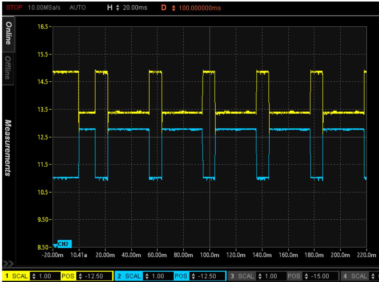
Figure 2-6. BQ76942 Cell Balancing With NPN BJT, Cell 4 (yellow) = 3.8 V, Cell 3 (blue) = 3.7 V
