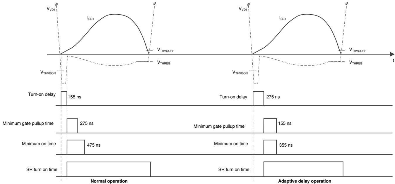
Figure 7. Adaptive Turn-on Delay
