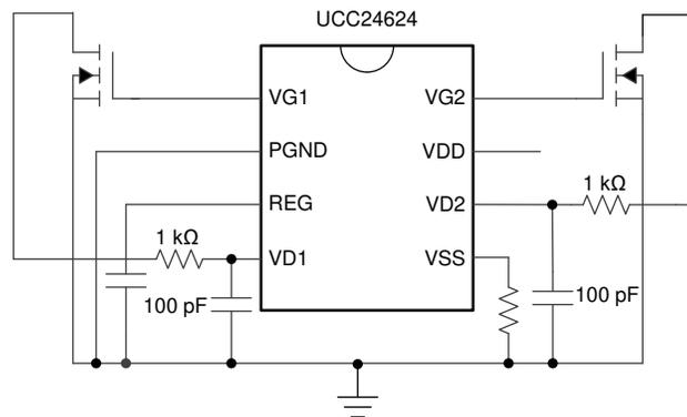
Figure 8. Adding RC Filter at VD Pins
