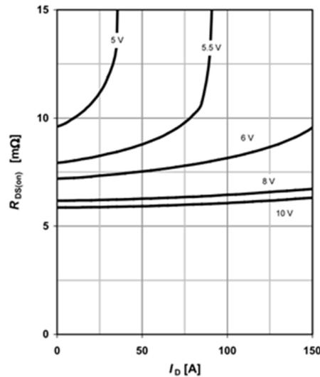
Figure 1. IPB072N15N3 Drain Source On-Resistance
