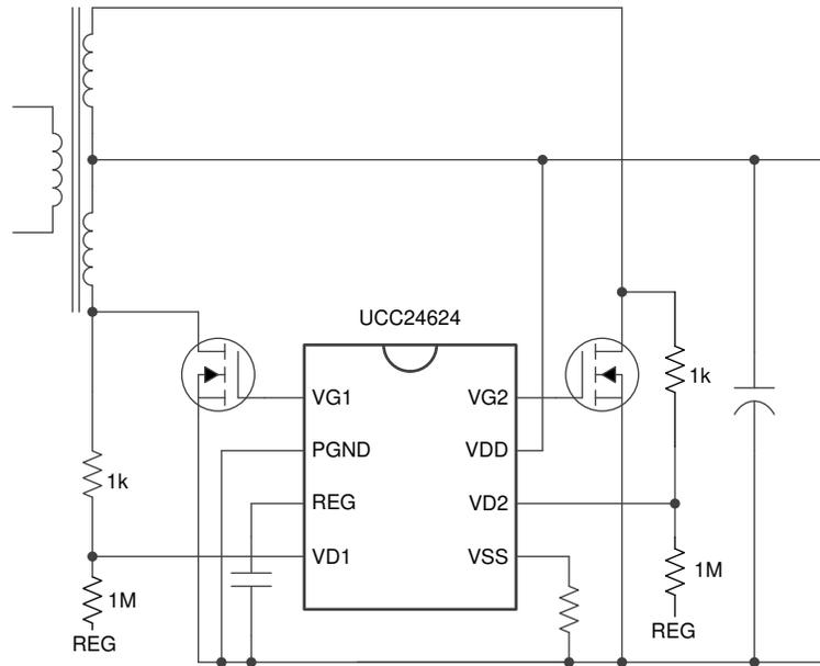
**Figure 6. Decreasing Turn-off Threshold Circuit**
