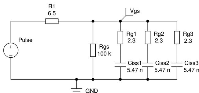
Figure 2. Driving Capability Simulation Circuit
