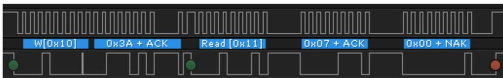
**Figure 1-4. Captured I2C Waveform for CC2 Current Reading**
