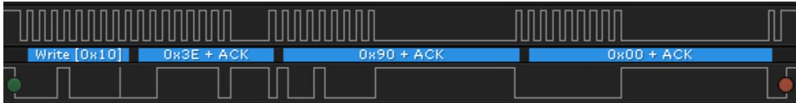
**Figure 3-2. Captured I2C Waveform for SET\_CFGUPDATE**
