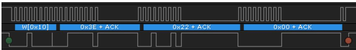
**Figure 2-3. Captured I2C Waveform for FET\_ENABLE Subcommand**
