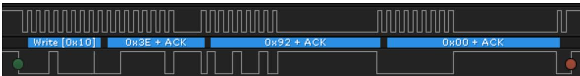
**Figure 3-5. Captured I2C Waveform for EXIT\_CFGUPDATE**
