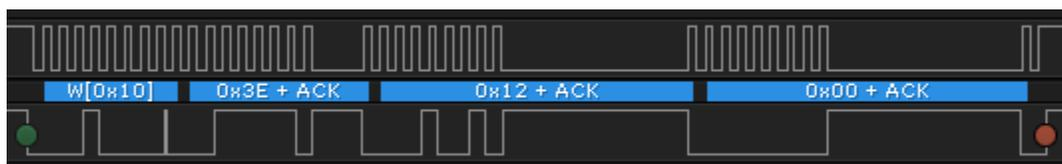
**Figure 2-4. Captured I2C Waveform of RESET Subcommand**
