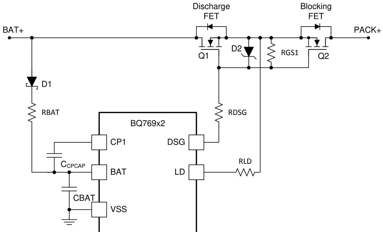
**Figure 17. Blocking Charge Current in the Discharge Path**
