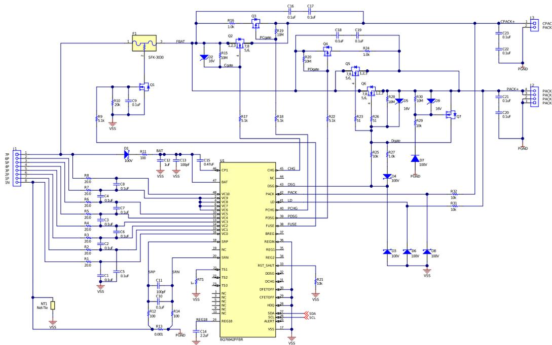
Figure 2. Typical 7S Parallel FET Schematic
