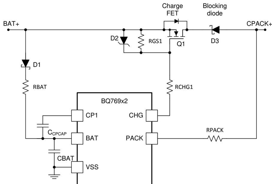
**Figure 9. Blocking Discharge in Charge Path with Schottky**
