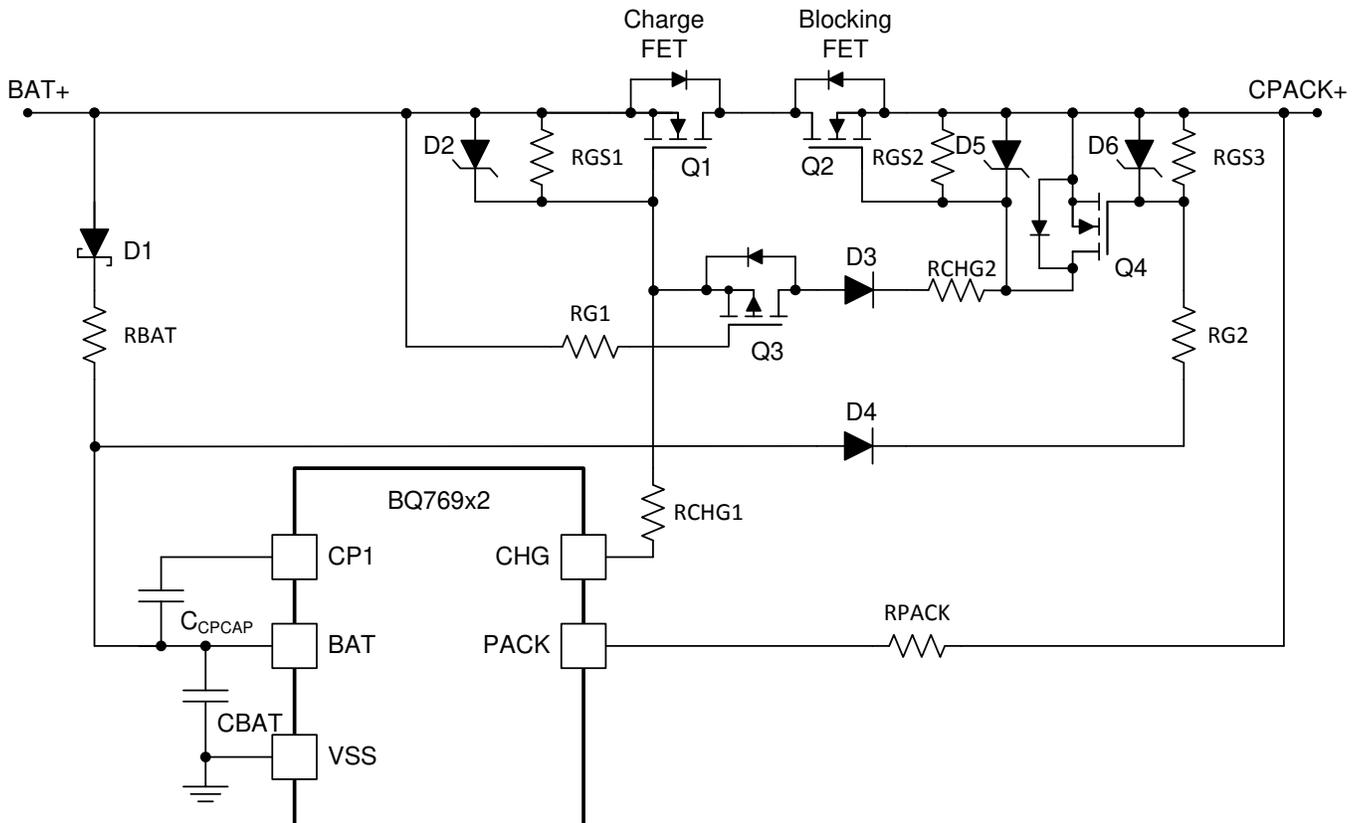
Figure 15. Charge Path with Blocking and Clamp FETs
