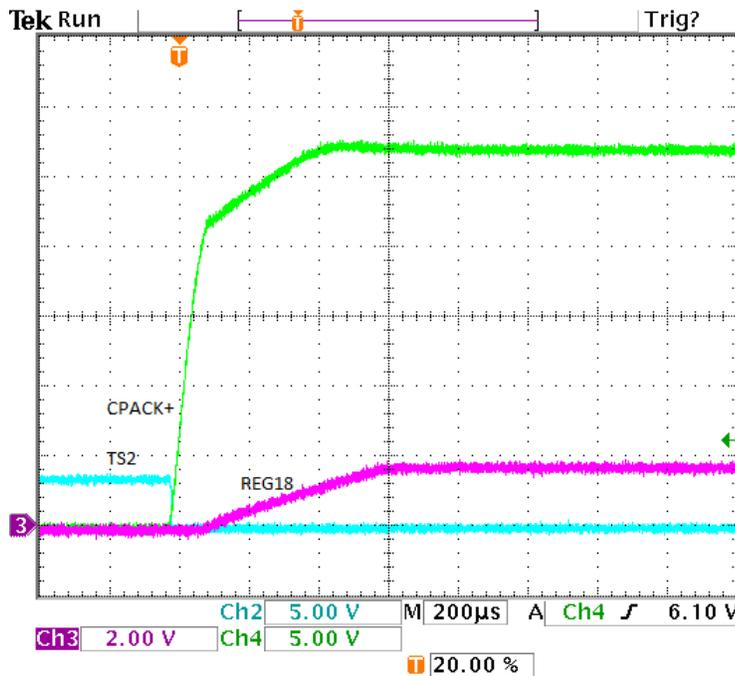
Figure 25. Wakeup from Charger Voltage
