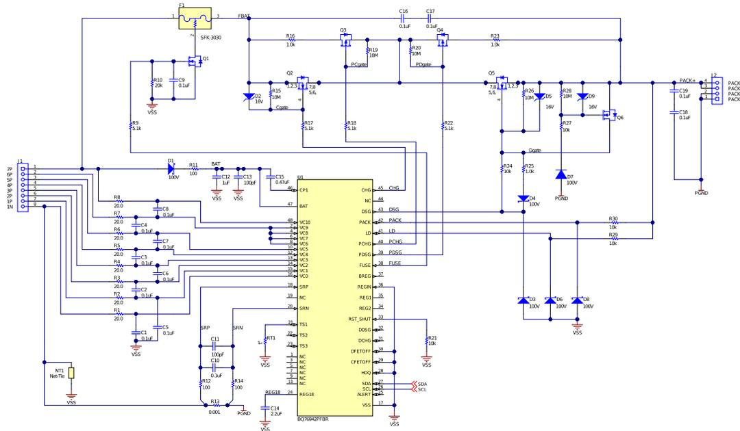
Figure 1. Typical 7S Series FET Schematic
