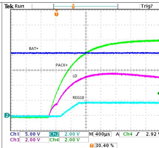
Figure 27. Wakeup from PACK+ Transient with Blocking FET
