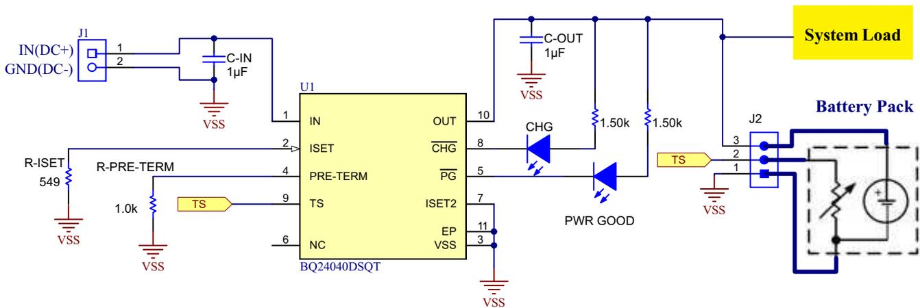
Figure 1. BQ24040 1-A Fast Charge and 5% Termination
