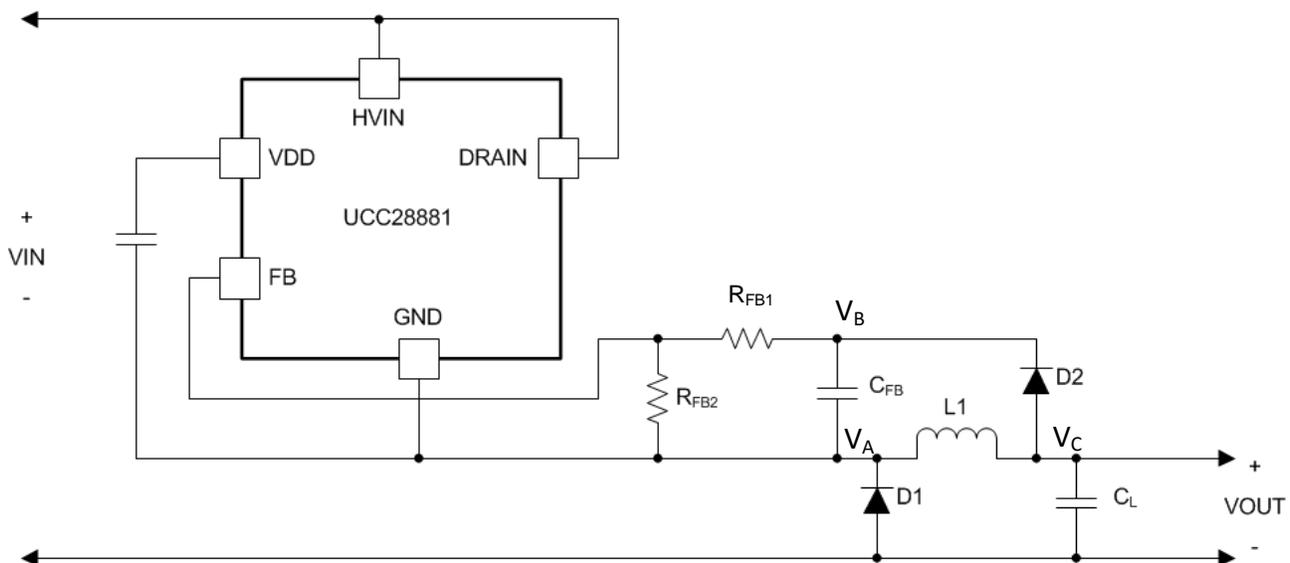
**Figure 1. UCC2888x High-Side Buck Converter Configuration**
