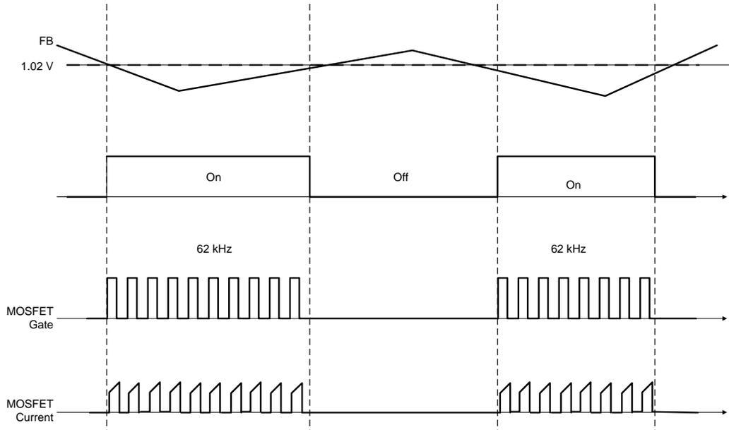
Figure 2. On/Off Control Diagram
