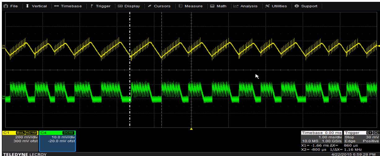
Figure 3. Output Ripple Voltage ( $V_{OUT} = CH1$ ) and Inductor Ripple Current ( $I_{L1} = CH4$ )
