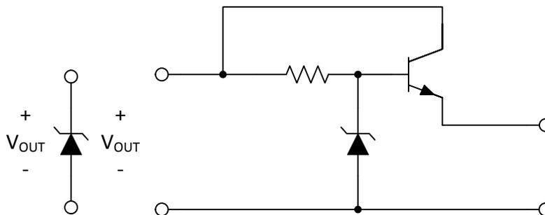
**Figure 4. Zener Shunt or Series Pass Regulator to Improve Load Regulation**
