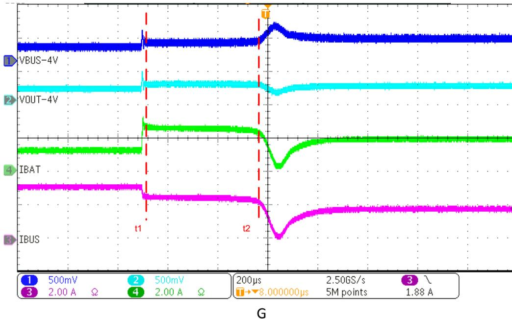
Figure 4.  $I_{BAT}$  Regulation Waveform
