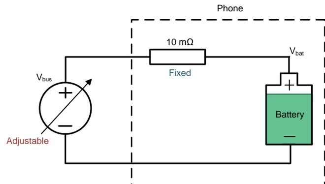
**Figure 2. Simplified Flash Charger Solution**
