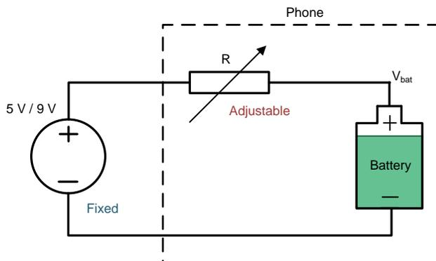
**Figure 1. Simplified Linear Charger Solution**
