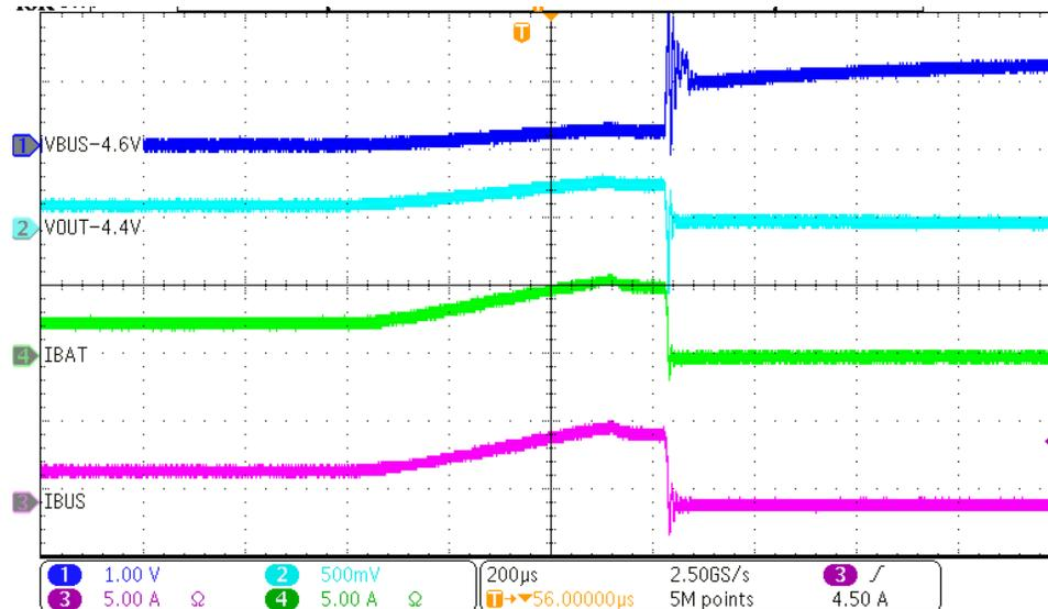
Figure 7.  $I_{BUS}$  OCP Waveform
