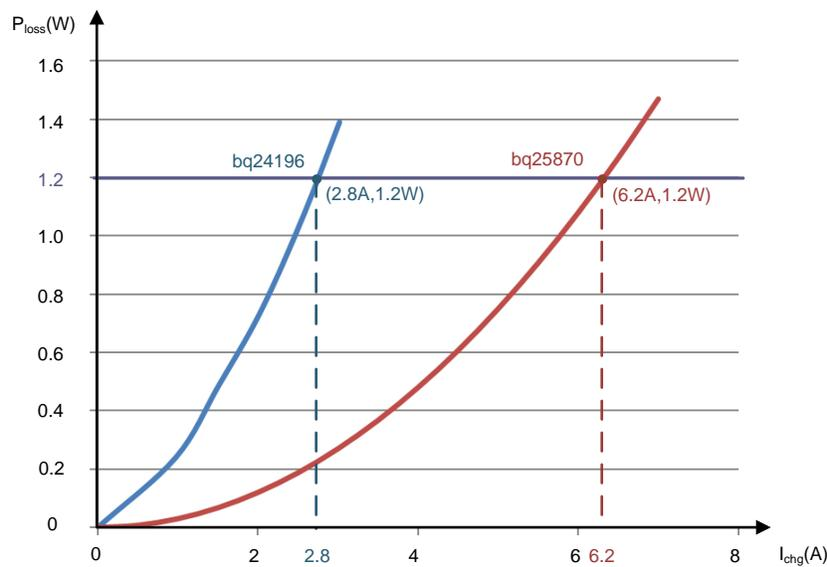
Figure 8. Power Loss Comparison Between Switching Charger and Flash Charger
