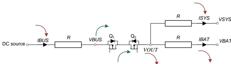
Figure 6. Simplified Circuit at  $t_2$
