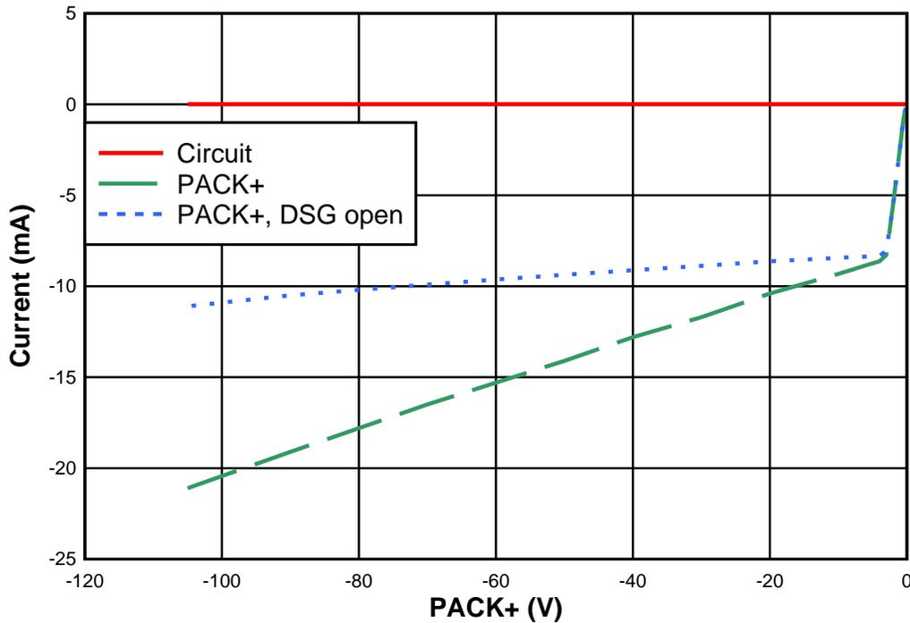
Figure 5. Test Circuit Currents With Reverse Voltage
