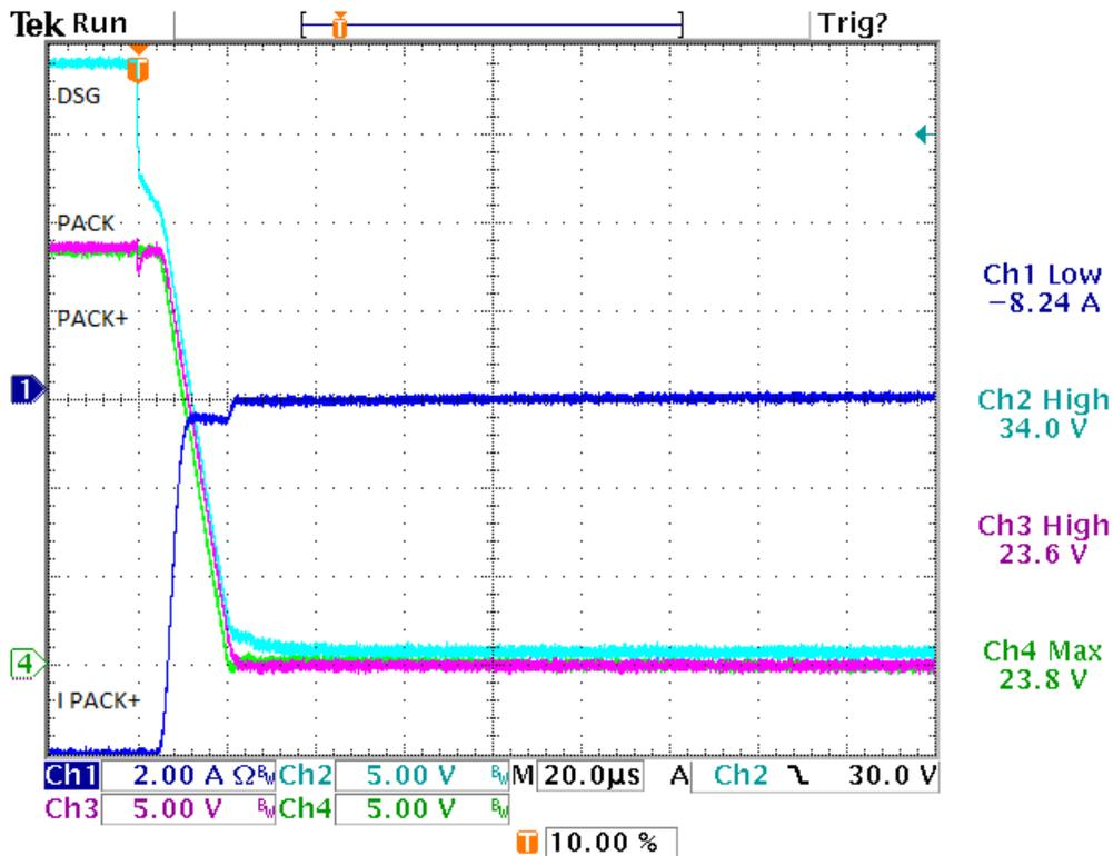
Figure 7. Turn Off With Reverse Voltage Circuit
