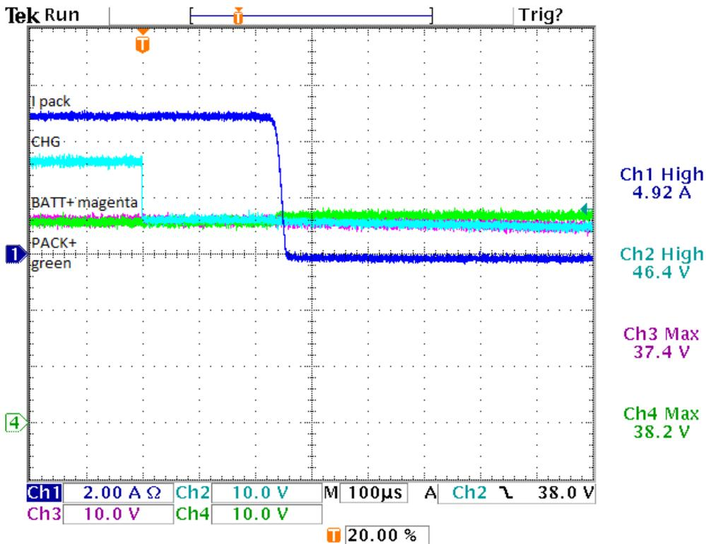
Figure 6. Charge FET Switching With Current Blocking Circuit
