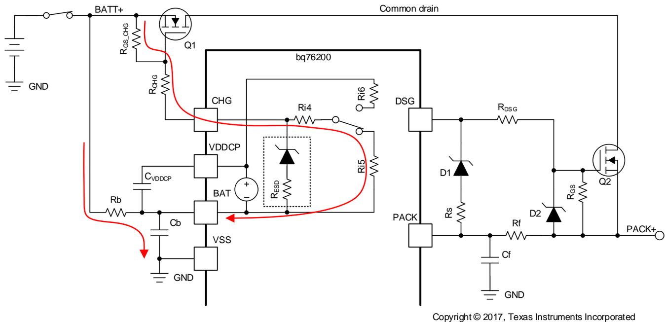
Figure 18. Battery Connection With Basic CHG Circuit
