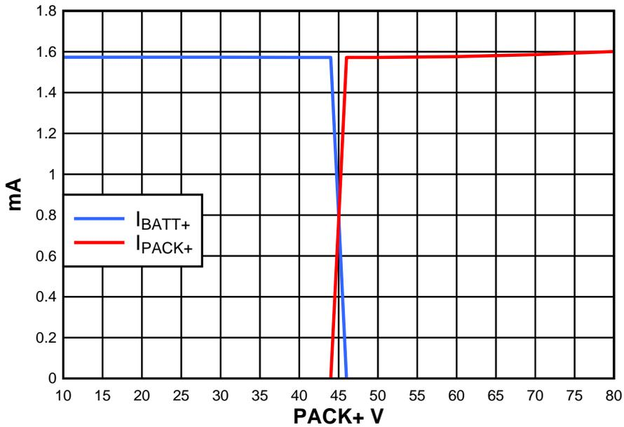
Figure 7. PACK Current From PCHGEN Example
