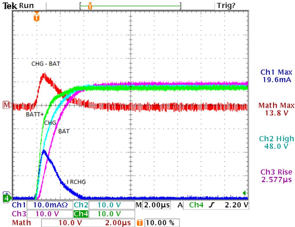
Figure 20. Battery Connection Example With D3, 510 Ω R<sub>CHG</sub>
