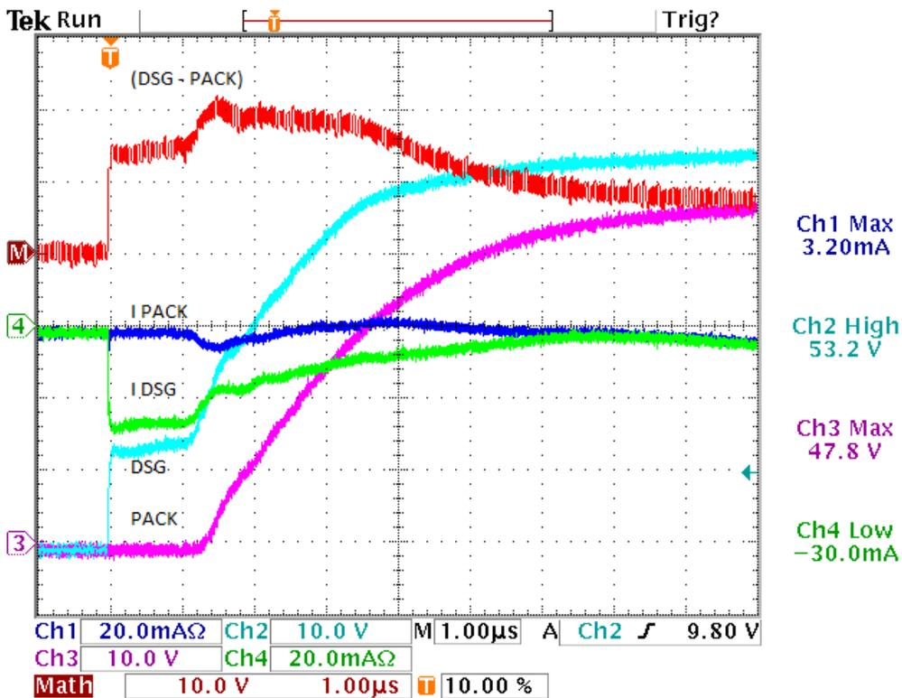
Figure 13. DSG Turn On With Resistor and Zener
