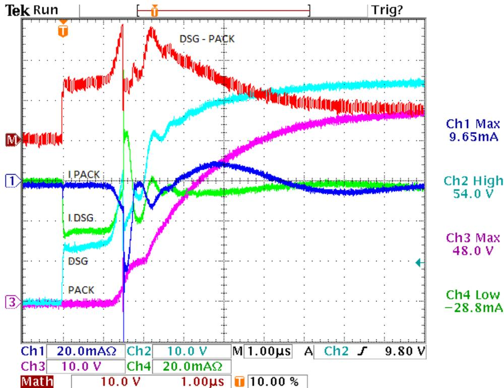
**Figure 11. DSG Turn On With ESD Trigger**
