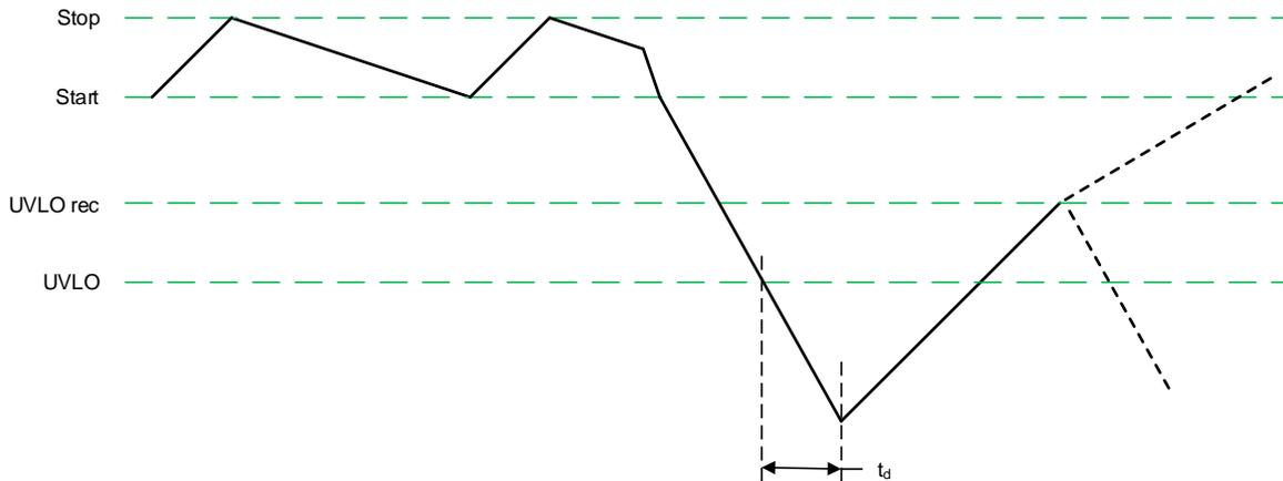
Figure 3. Charge-Pump Thresholds
