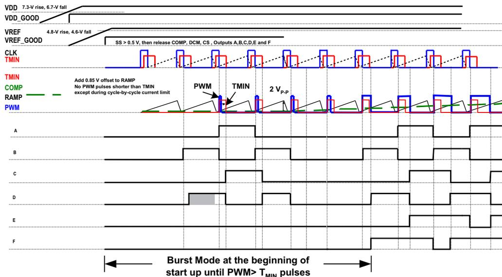
**Figure 1. UCC28950/UCC28951-Q1 Startup and Burst Mode Timing Diagram (The Area in Grey is Not Ensured)**
