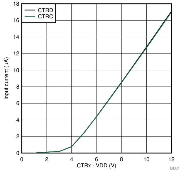
**Figure 3-2. Example CTR<sub>x</sub> pin Characteristic**
