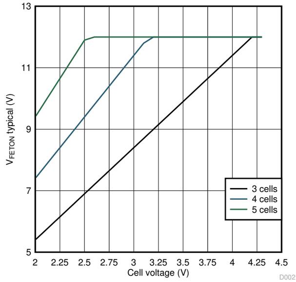
**Figure 3-4. FET Drive Voltage With Cell Variation**
