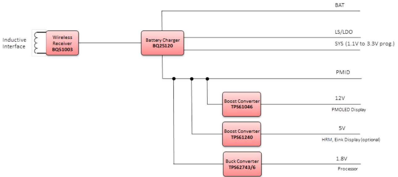
Figure 2. Block Diagram of Wearable Power Management
