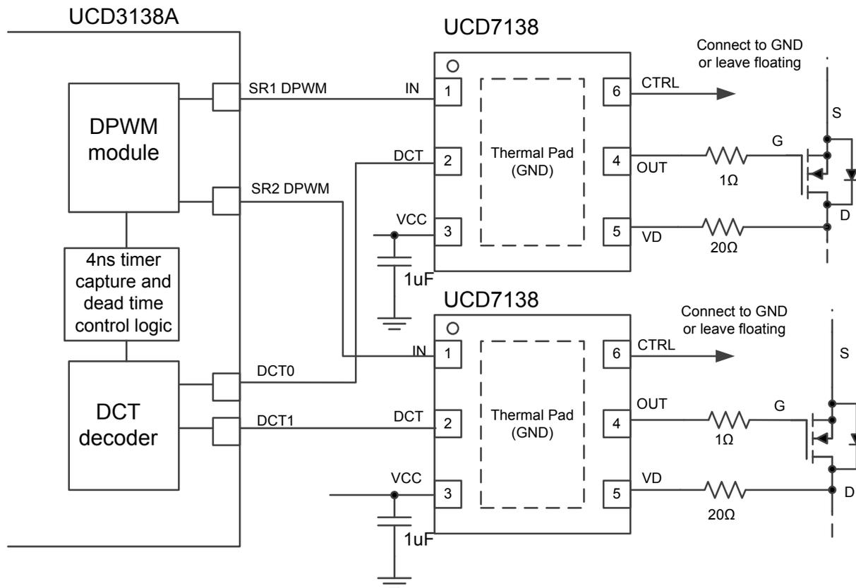
**Figure 3. Low Side Gate Driver with Body Diode Conduction Sensing**
