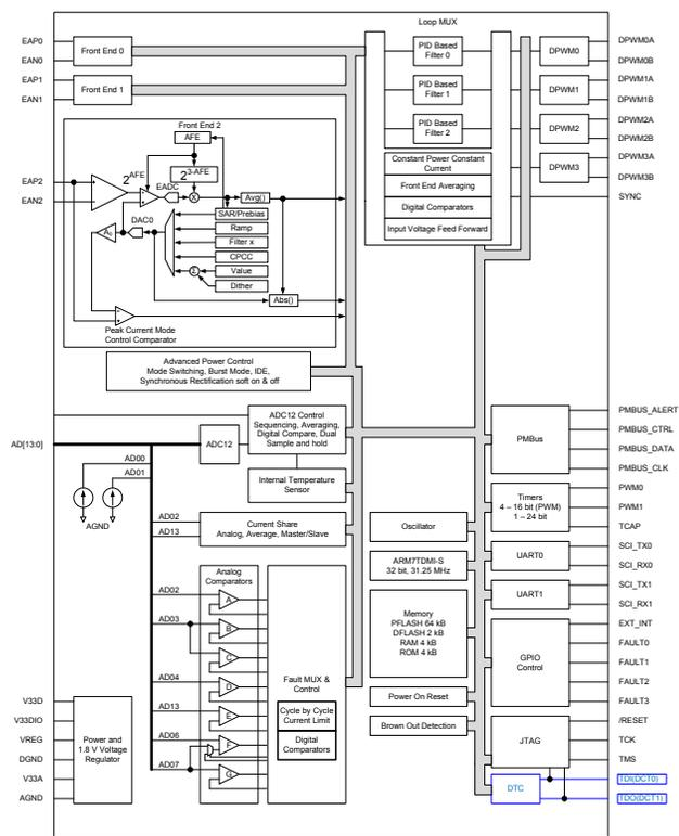
**Figure 2. UCD3138A Block diagram**
