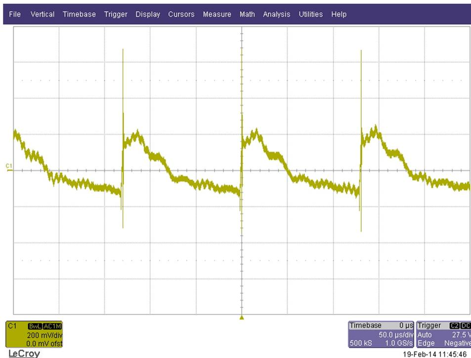
Figure 20. Vout Ripple at Vin = 275 VAC, Full Load
