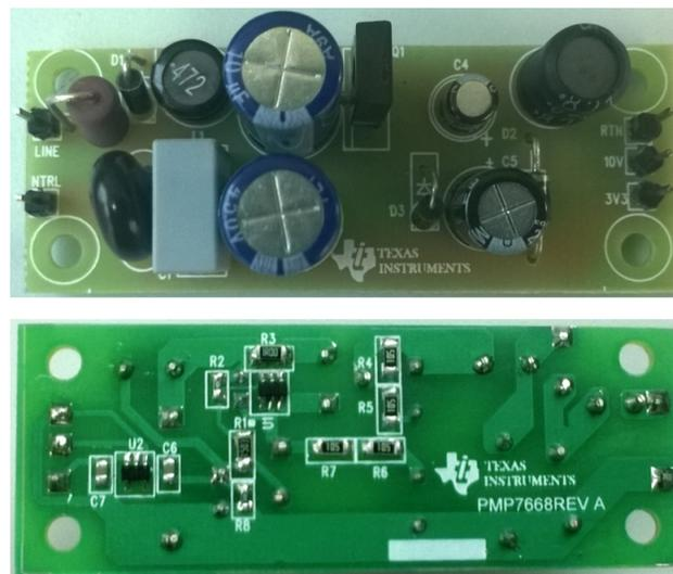
Figure 1. AC-DC Buck Design Using UCC28722 (PMP7668)
