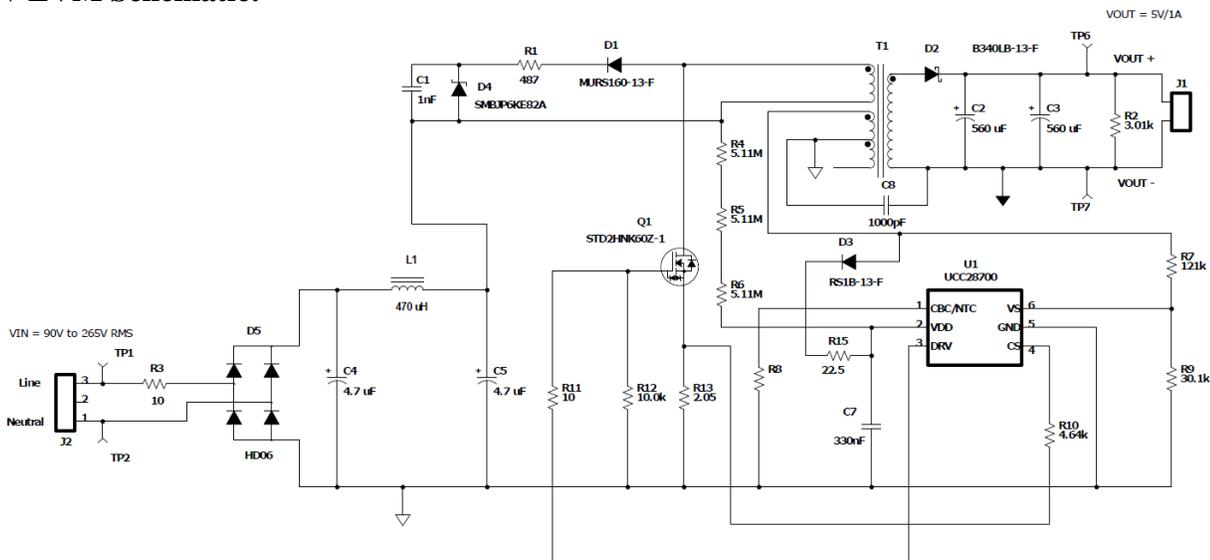
Figure 7, Schematic
