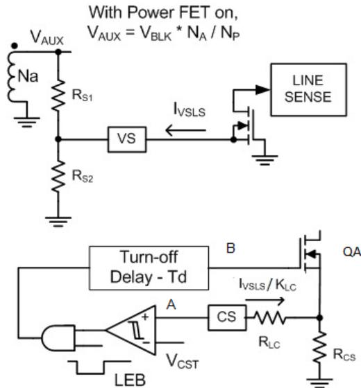
Figure 5, Peak Current Limit Comparator
