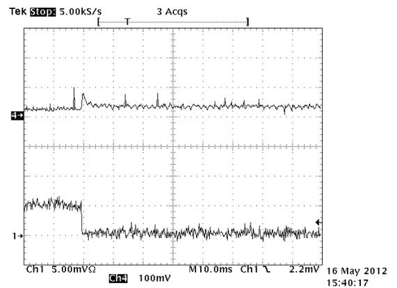
Figure 10, 0.6 to 0.1A load step
