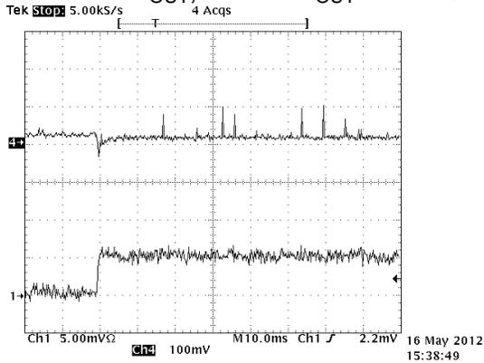
Figure 11, 0.1 to 0.6A load step
