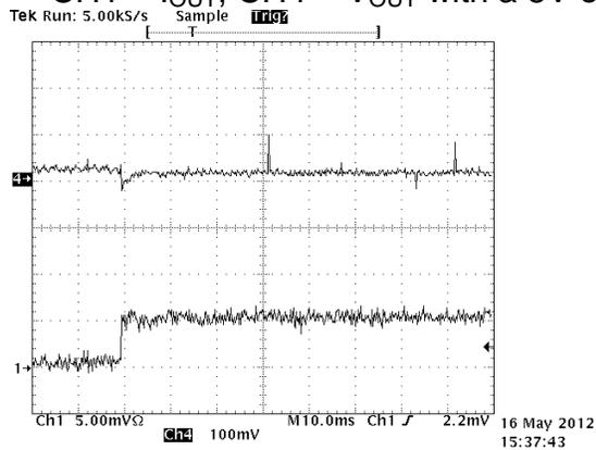
Figure 9, 0.1 to 0.6A load step
