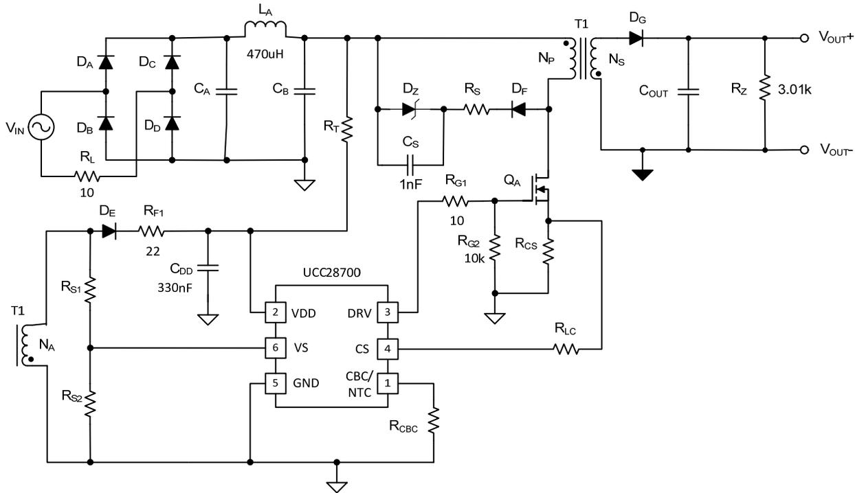
Figure 1, UCC28700 5W Offline Flyback Functional Schematic
