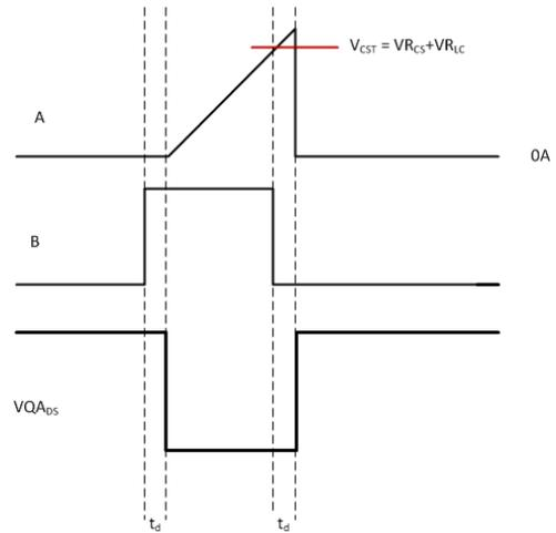
Figure 6, CS(A), QA<sub>g</sub>(B), VQA<sub>DS</sub> Signals
