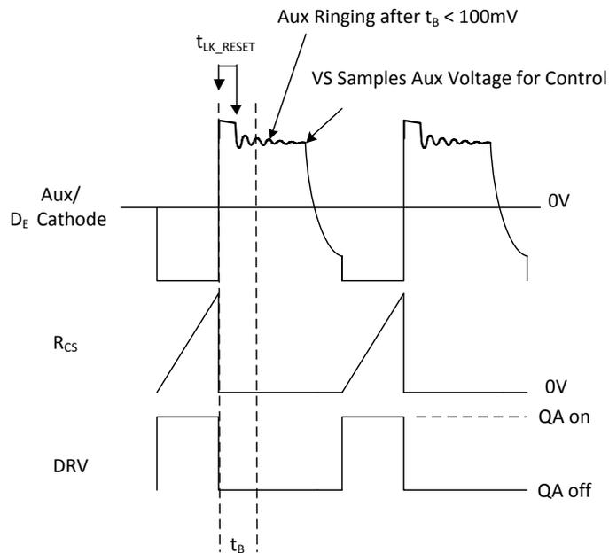
Figure 4, Auxiliary Winding VS Blanking
