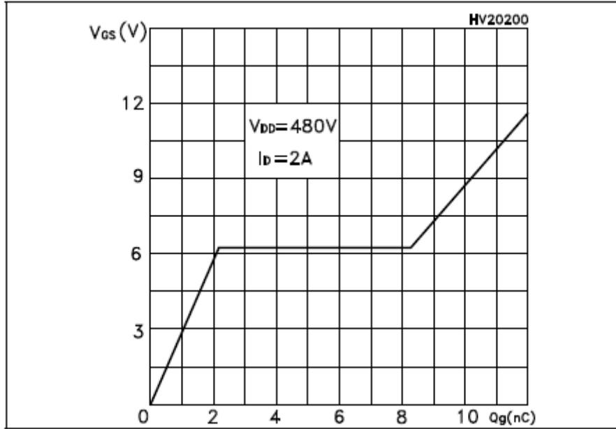
Figure 3, Gate Charge vs  $V_{gs}$
