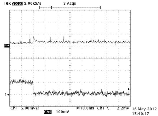
Figure 12, 0.6 to 0.1A load step
