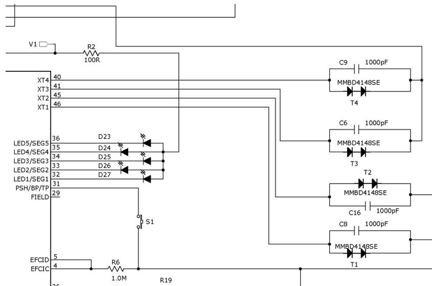
**Figure 10. LED-Based SOCi Indicator Circuit Using bq78PL114S12 With FW5000**
