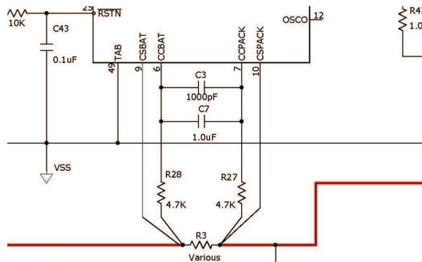
Figure 6. Current Measurement Circuit
