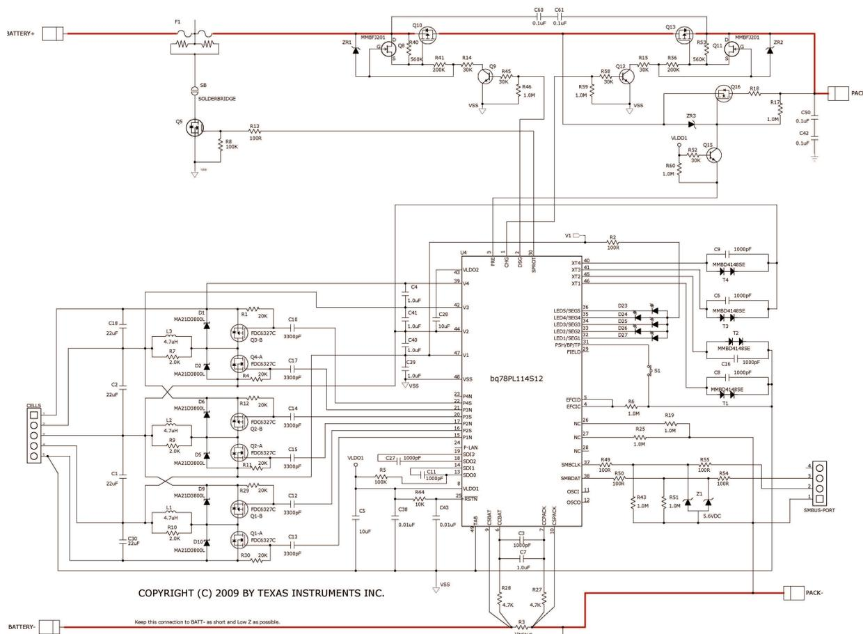
Figure 24. Reference Design With Four Cells and bq78PL114S12 (FW5000)
