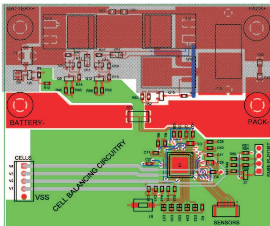
**Figure 14. VSS Star Ground and Internal Copper Plane**
