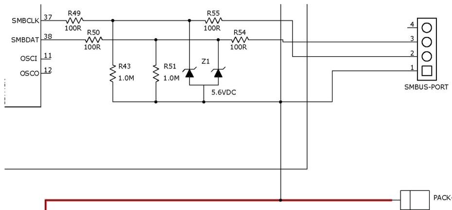
Figure 12. SMBus Interface Circuit
