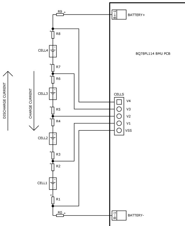
**Figure 3. Schematic of Battery Sense Connections and System Impedances**
