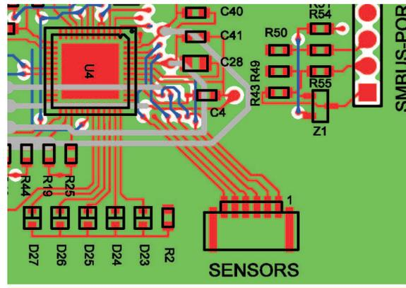
Figure 16. Layout of Temperature Sensor Signals
