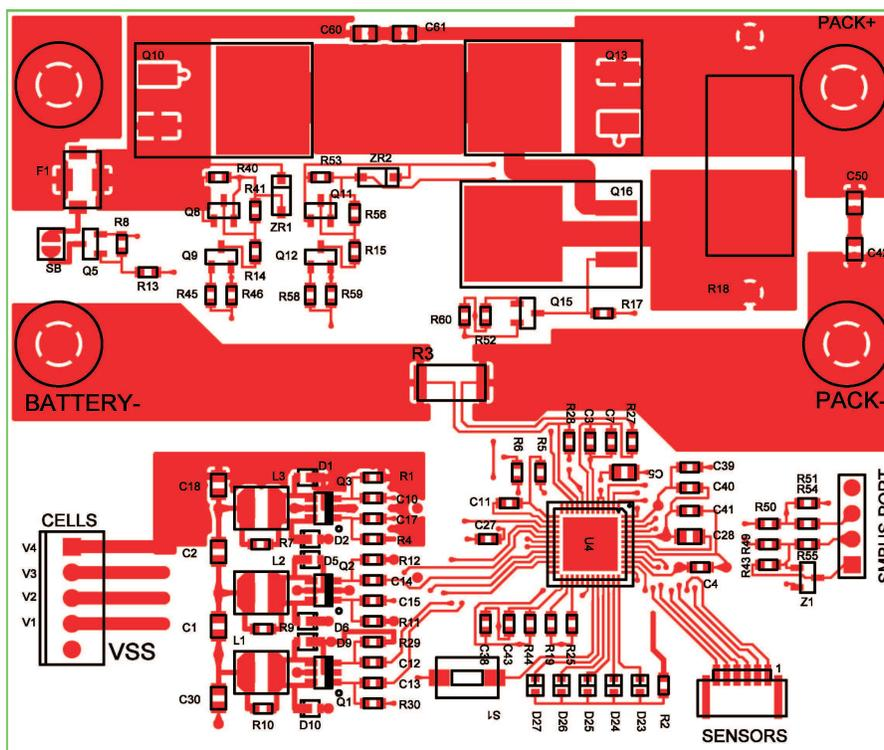
Figure 18. Top Layer of Finished Design
