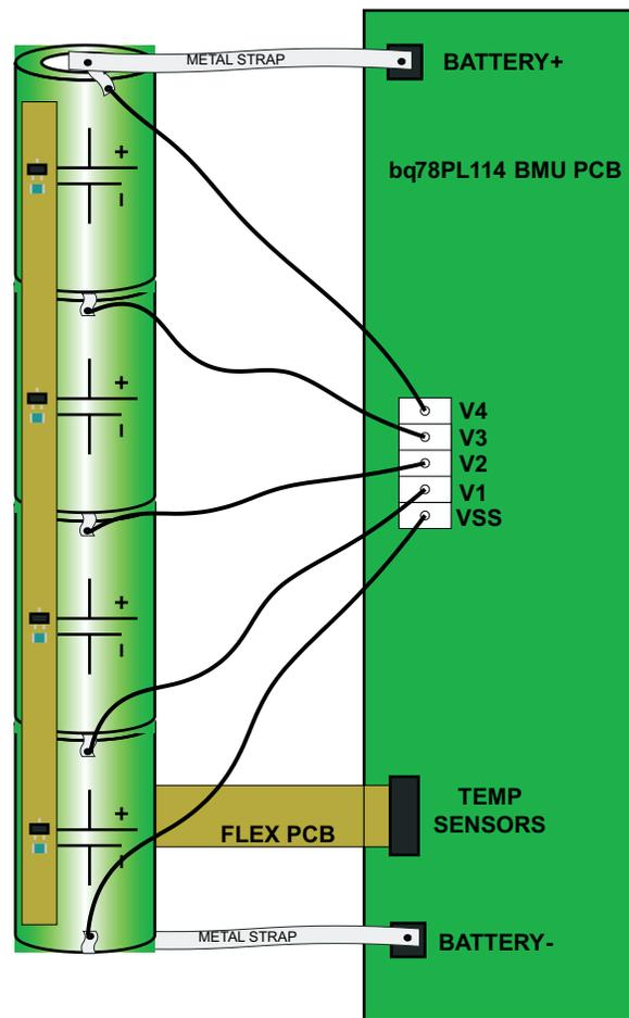
**Figure 1. Battery to BMU Power, Cell Voltage, and Temperature Connections**
