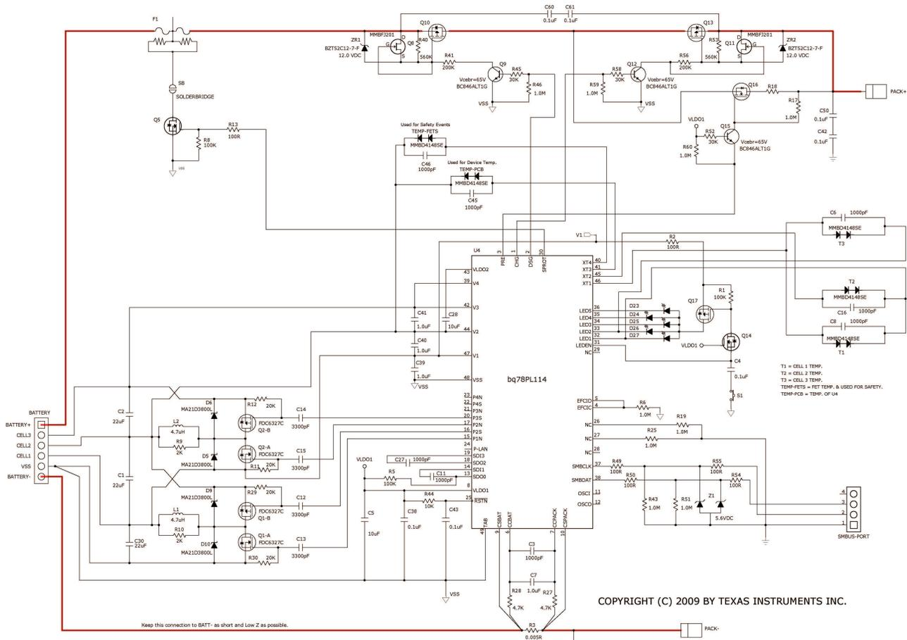
Figure 23. Reference Design With Three Series Cells and FW4452
