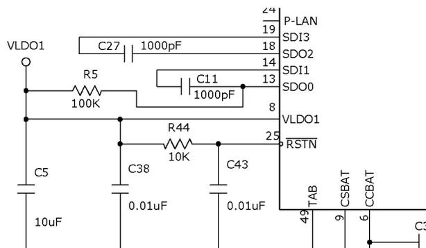
**Figure 5. PowerLAN™ Circuitry**
