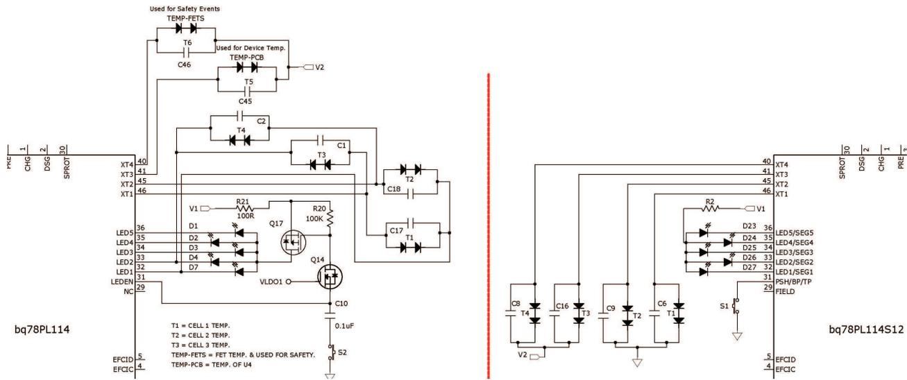
Figure 11. Temperature Sensor Multiplexing vs Nonmultiplexing (S12)
