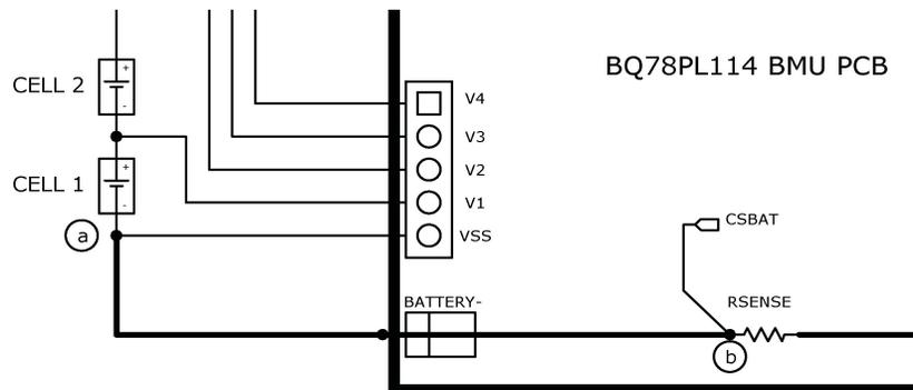
**Figure 2. Battery-Connection Voltage Drop Requirements:  $V_{ab} < 100$  mV During Charge**
