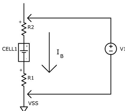
**Figure 4. Effect of Impedance on V1 Voltage Measurement**
