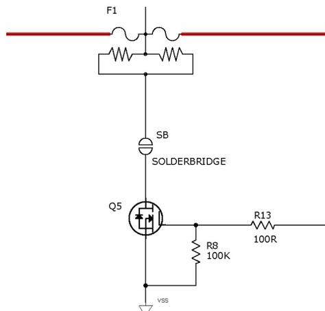
Figure 8. Chemical Fuse Circuit
