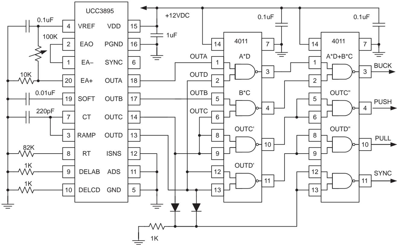
Figure 5. Circuit Implementation Using NAND Gates
