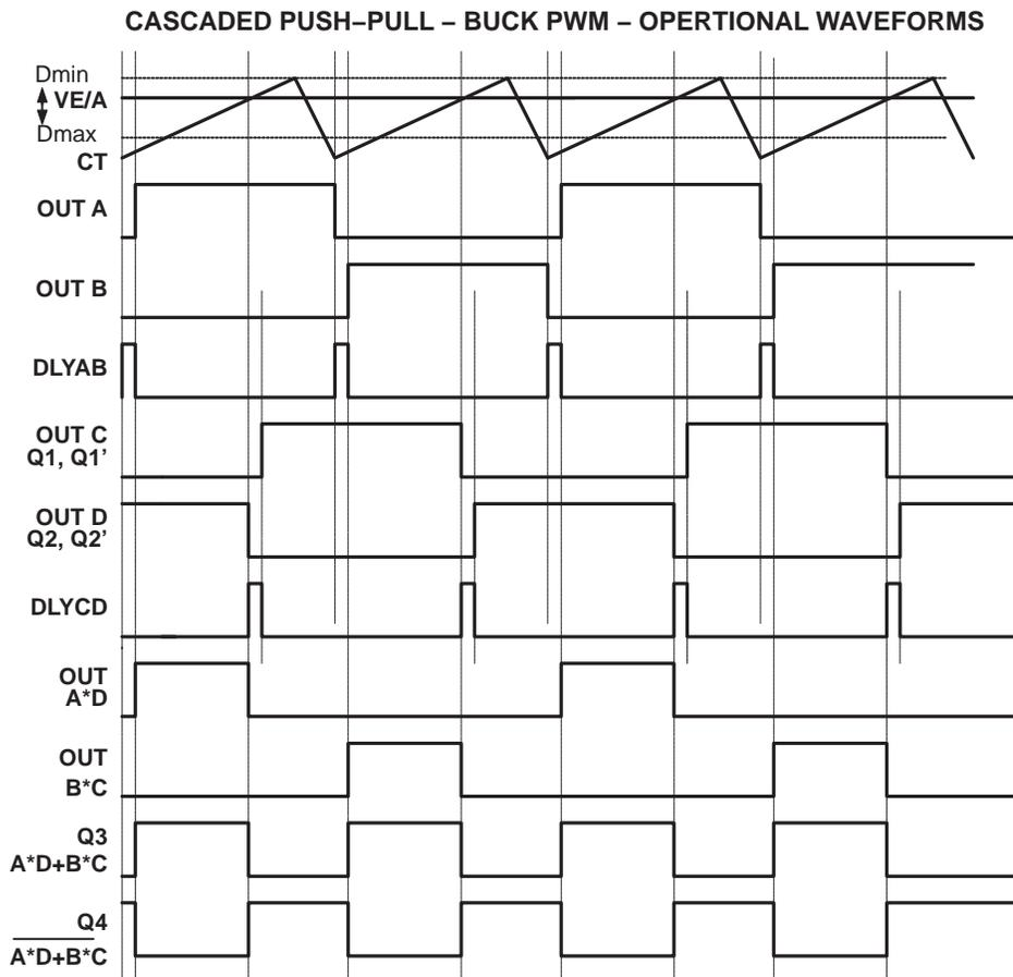
Figure 2. Operating Waveforms
