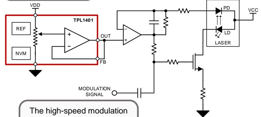
The high-speed modulation DAC need not take the load of controlling the biasing dynamically
