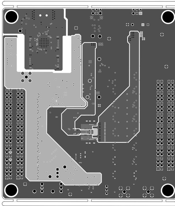
**Figure 5-17. PCB Layer 9 (Ground 5/Power 2)**
