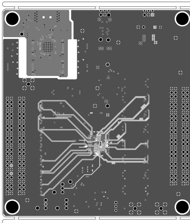
**Figure 5-18. PCB Layer 10 (Signal 6)**
