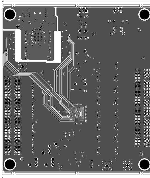
**Figure 5-11. PCB Layer 3 (Signal 1)**
