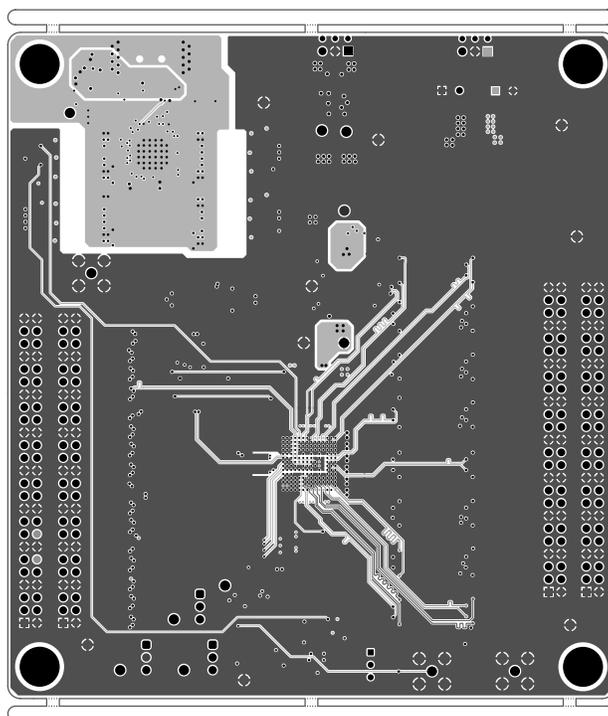
**Figure 5-14. PCB Layer 6 (Ground 3/Signal 3)**
