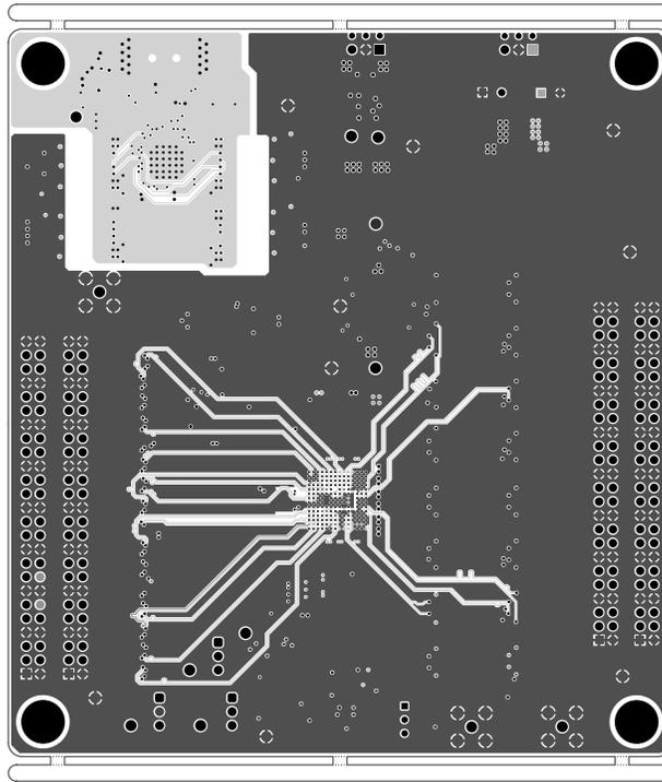
**Figure 5-15. PCB Layer 7 (Ground 4/Signal 4)**
