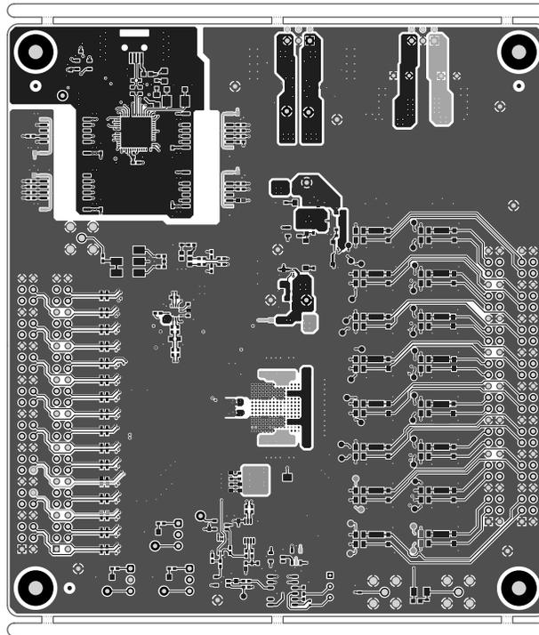
**Figure 5-9. PCB Layer 1 (Top Assembly Drawing)**
