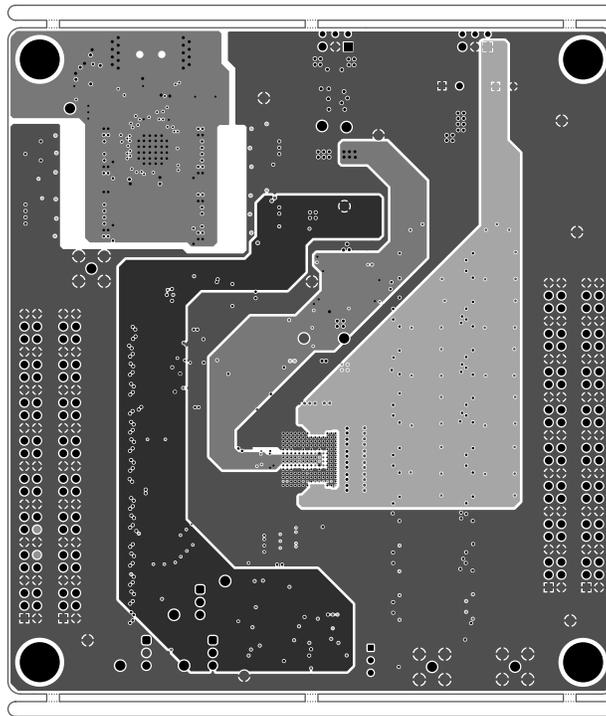
**Figure 5-12. PCB Layer 4 (Ground2/Power 1)**
