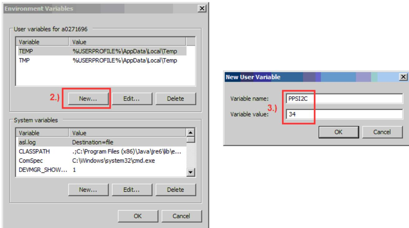
**Figure 9. Environment Variable and User Variable Window**
