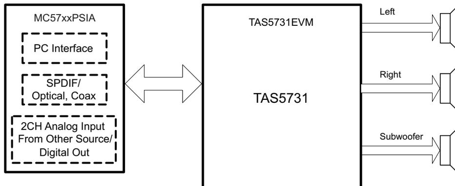
**Figure 2. Complete System and EVM Signal Path Overview**
