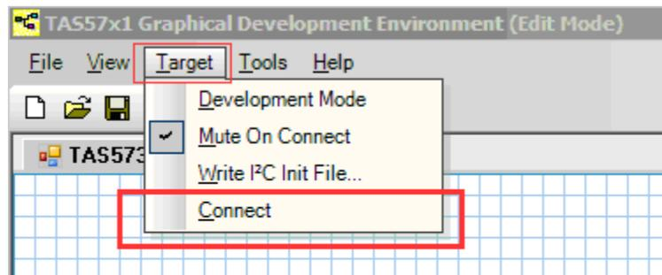
**Figure 12. Initiating Connect from the Target Menu**
