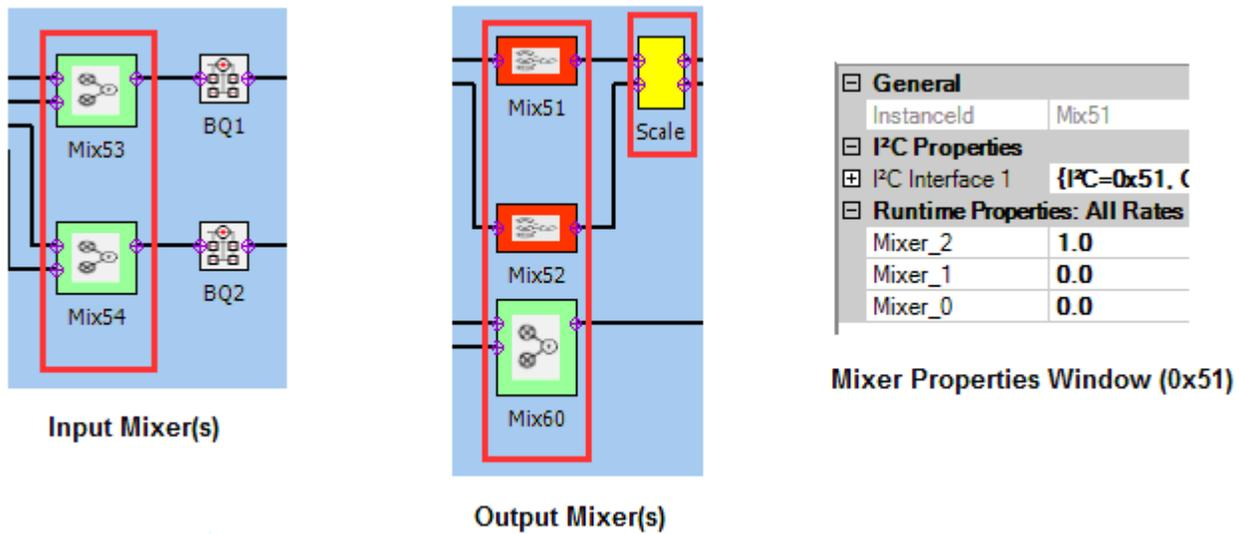
Figure 19. Input, Output Mixer and Scaler Nodes
