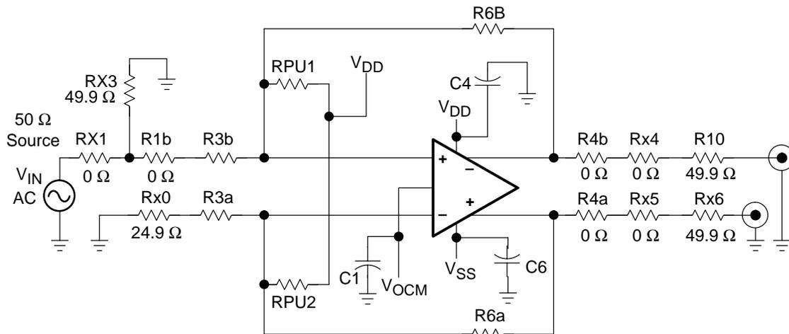
**Note:** Shifting the VICR within the specified range in the data sheet via RPU1 and RPU2 if the VICR is out of the specified range. See the Application section of the data sheet for the THS4121 for more information.
