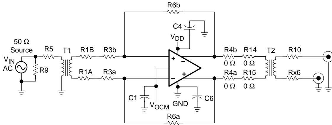
**Note:** Utilizing the input and output transformers to create a fully-differential signal input/ differential or single output and isolate the amplifier from the rest of the front-end and back-end circuits.
