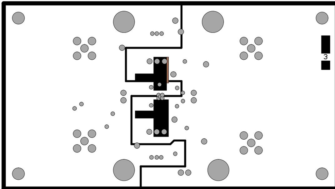
Figure 1–11. Bottom (Layer 4) (Ground and Signal)
