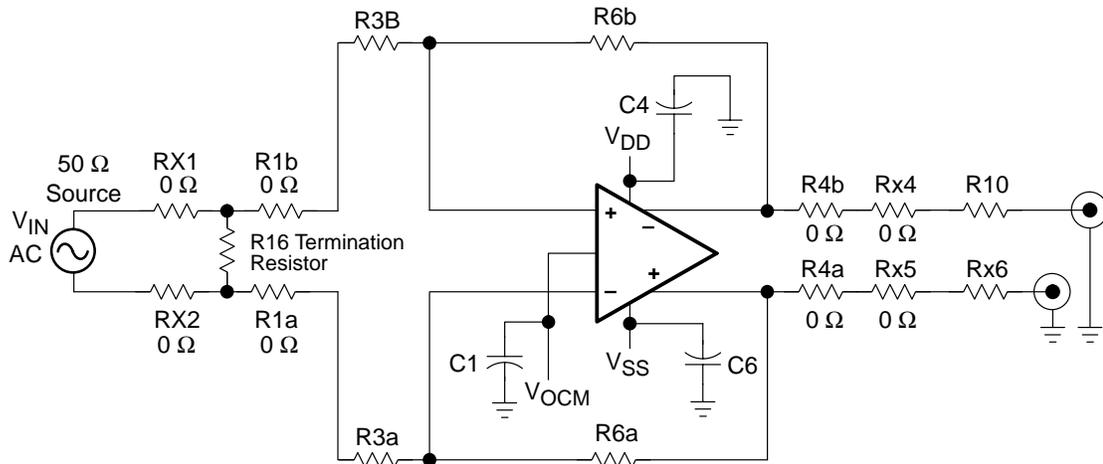
**Note:** Fully-differential in / fully-differential out signal path. See the *Texas Instruments February 2001 Analog Applications Journal* for the information on the termination resistors.
