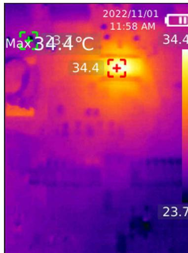
**Figure 2-6. DRV8462, DDW Package, Auto-Torque Enabled**
