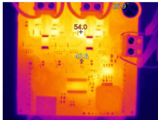
**Figure 2-9. DRV8711 Thermal Image at 50 V, 3A, 1/8 Microstep, 1 kpps**
