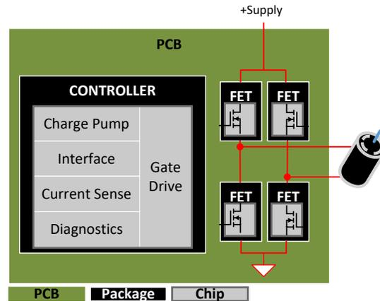
**Figure 1-1. Gate Driver With External FETs**
