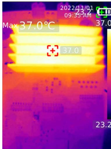
**Figure 2-8. DRV8462, DDV Package, Auto-Torque Enabled**
