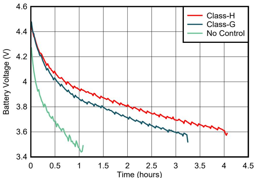
**Figure 3-13. Battery Life: Class-H, Class-G, and No Control**
