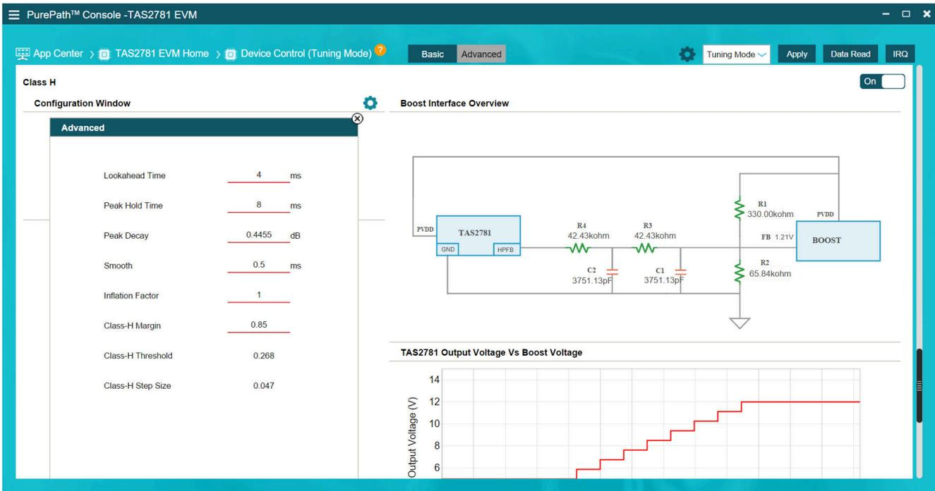
Figure 3-3. Class-H Advanced Controls
