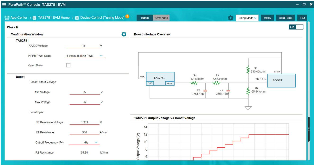
Figure 3-2. Class-H Controls in Device Control Page
