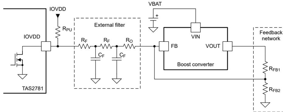
**Figure 3-1. Hardware Connections**
